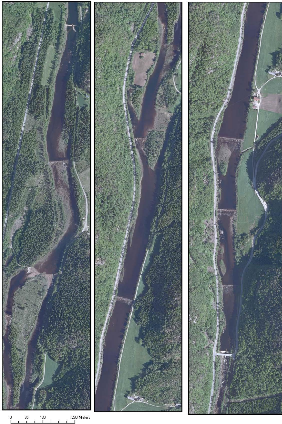
Annex 2. Laudal Bypass section in Mandalselva River under a discharge of 3 m 3 /s on the 30/05/2009.
