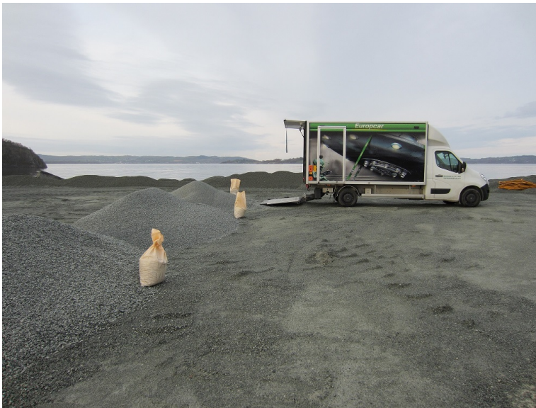
Figure 3.1: Transporter and piles of crushed aggregate 4/8 mm, 8/11.2 mm and 14/16 mm.
