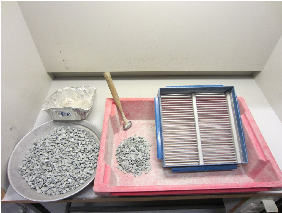
Figure 2.8: Particle size 8/10 mm being screened by 5 mm bar sieve.
