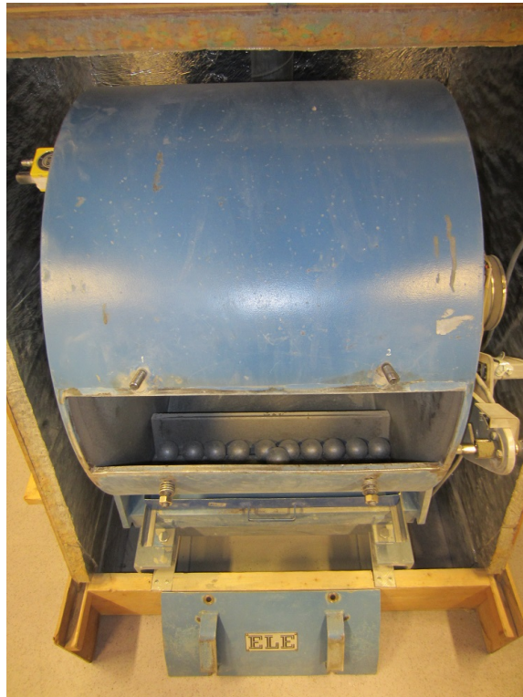
Figure 2.2: Los Angeles test machine used in study.
