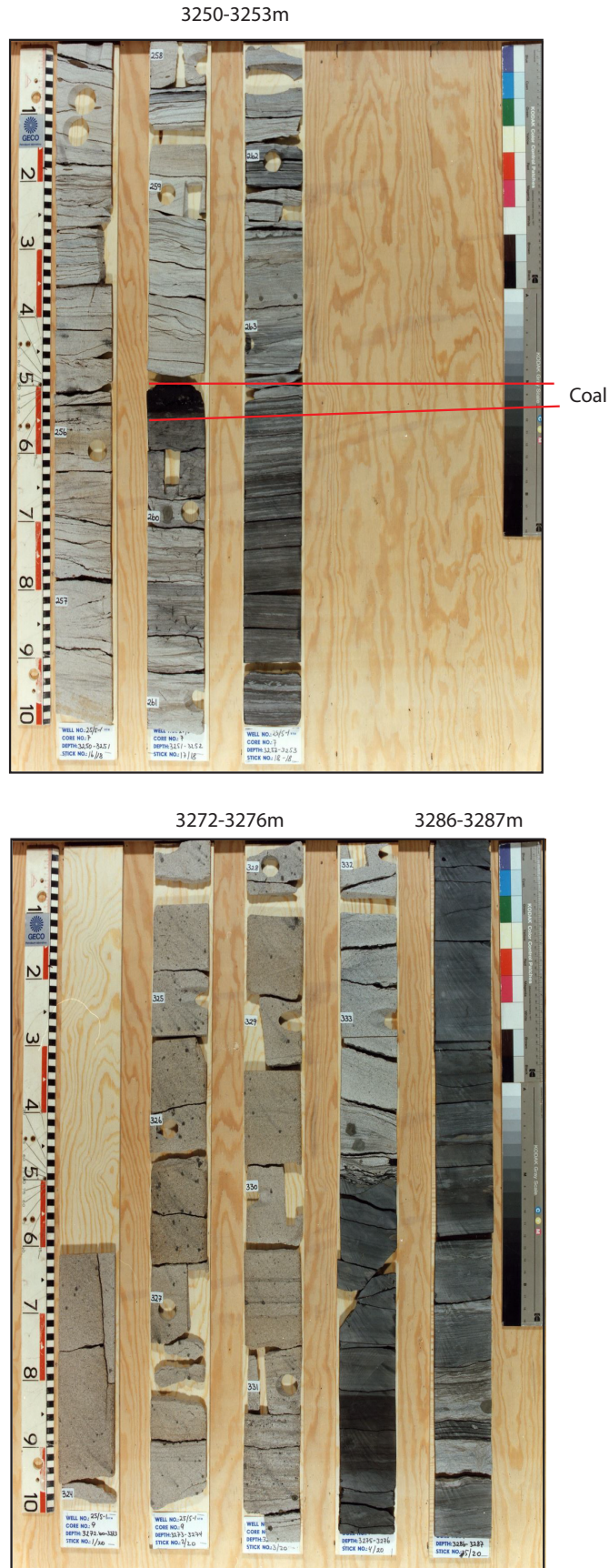
Fig. 6.10 Core photos well 25/5-1. 3250-3253m = coal at 3250. 3272-3276m, 3286-3287 = transition between upper fine sandstones and shales to upper coarse sandstone. Photos from NPD
