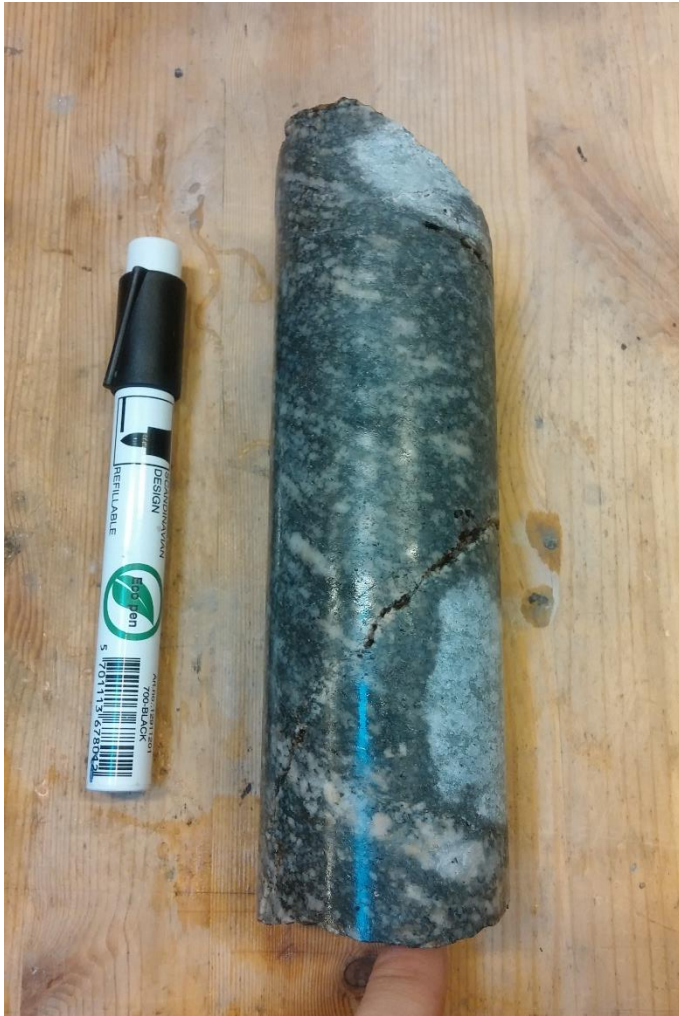
Figure 6.3 - Core #5 with discontinuity plane
