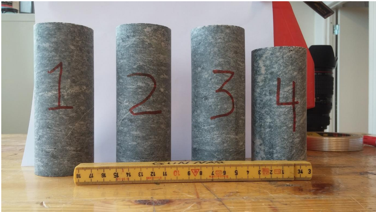
Figure 6.4 - Core samples 1-4 after sample preparation
