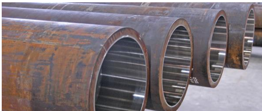
Figure 1 - Clad pipes prior to girth welding.[5]
