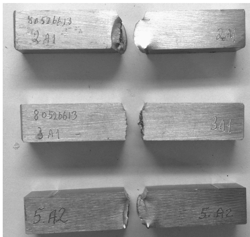
Figure 18. Charpy V-notch specimens of all three welds.
