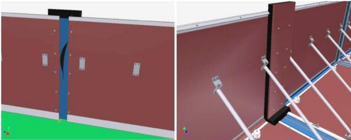
Picture 14: Damaged and repaired PVC canvas.
