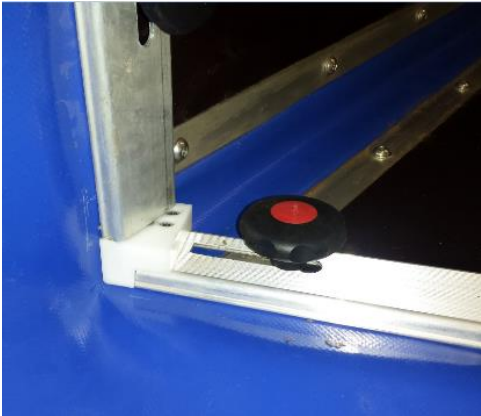
Picture 4: Canvas from the first panel (to the left) secured by the canvas clamp on the second panel
