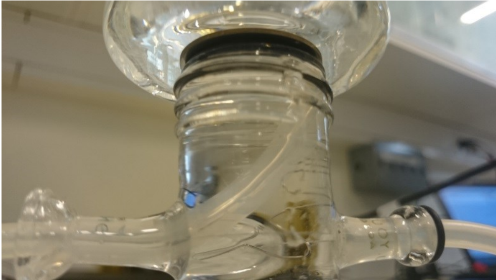
Figure 3.13 View of the tubes performing the suction in the first setup
