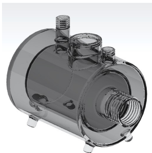
Figure 4.26 After interaction with the glass blowers, alterations were made to the double walled cell
