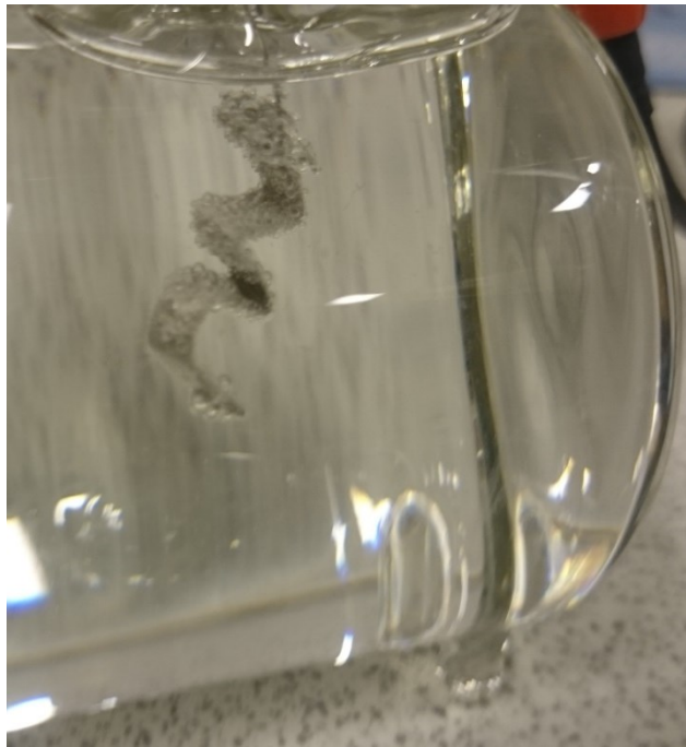
Figure 3.18 Counter-electrode after trying to use flow to remove bubbles
