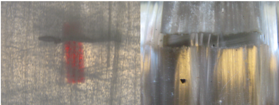
Figure 3.7: The left image shows a visible compressive crack of fibres at the location of impact, on the outside of the pipe. The right image shows that the fibres are broken in this area, and that the damage extends through the entire hoop layer. The red rectangle is a strain gauge used to measure strain during impact.
