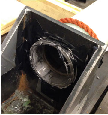
Figure 8.5: Jig for separating pipe from mandrel.
