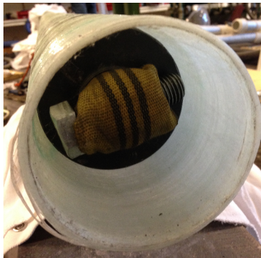
Figure 8.6: Strap is secured to the plate, then pulled through.
