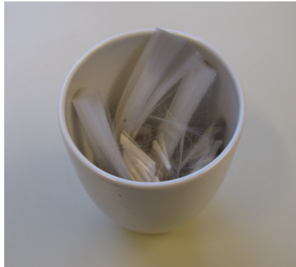
Figure 3.5: Fibres of a sample after burn-off.
