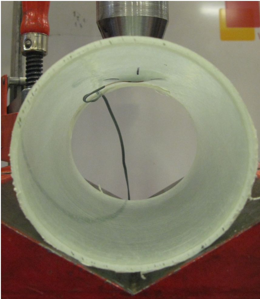
Figure 3.9: Pipe being impacted while strain is continuously measured.
