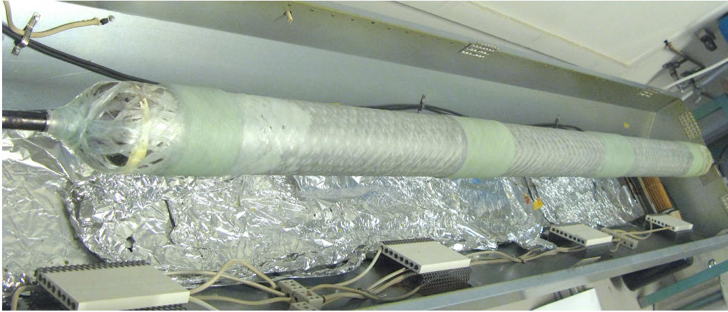
Figure 3.8: \pm 55^\circ Pipe in curing oven, note fibre patches distributed along the pipe
