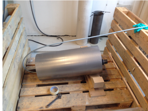
Figure C.2: Composite tube inside metal shield during testing
