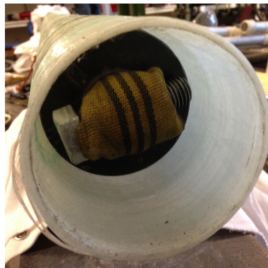
Figure F6: Strap is secured to the plate, then pulled through.
