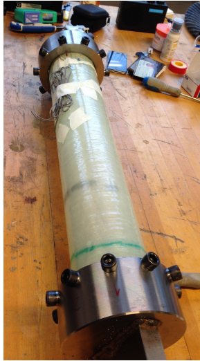
Figure C.1: A composite tube with end-fittings attached ready for pressure testing
