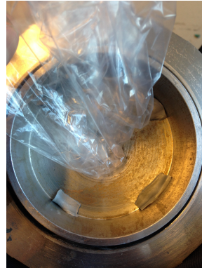
Figure C.4: Plastic liner method before assembly
