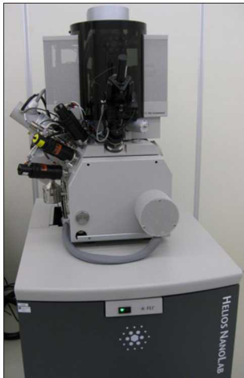
Figure 4.2: Picture of the FIB used in this project. The FIB is located at the NTNU Nanolab [23].
