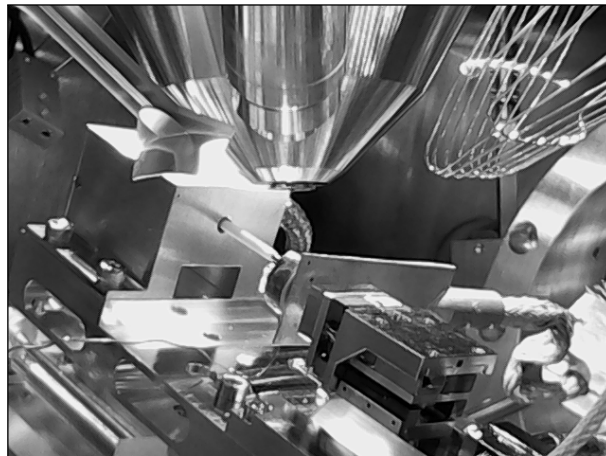
Figure 6.4: Picture of the indenter equipment installed in the SEM [26]
