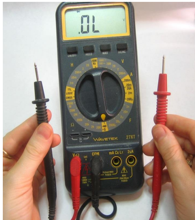
Figure 37 Multimeter used to measure the conductivity
