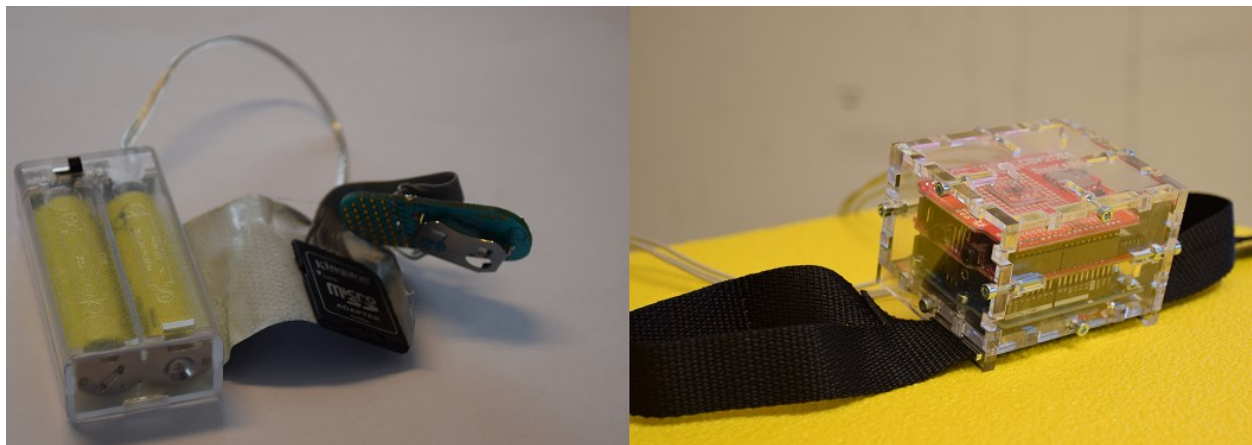
Figure 2.2: Bean setup (left) and Arduino Uno setup (right)
