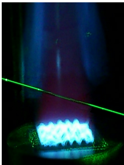
Figure III.1: Photograph of laminar premixed CH 4 -air flat flame (PF-CH 4 -air-3).
