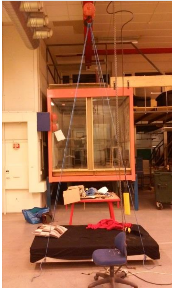
Figure 4-1 Experiment set-up. Mattress hanging from ceiling crane
