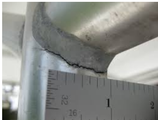
Figure 1.1: A tubular joint with crack developing
