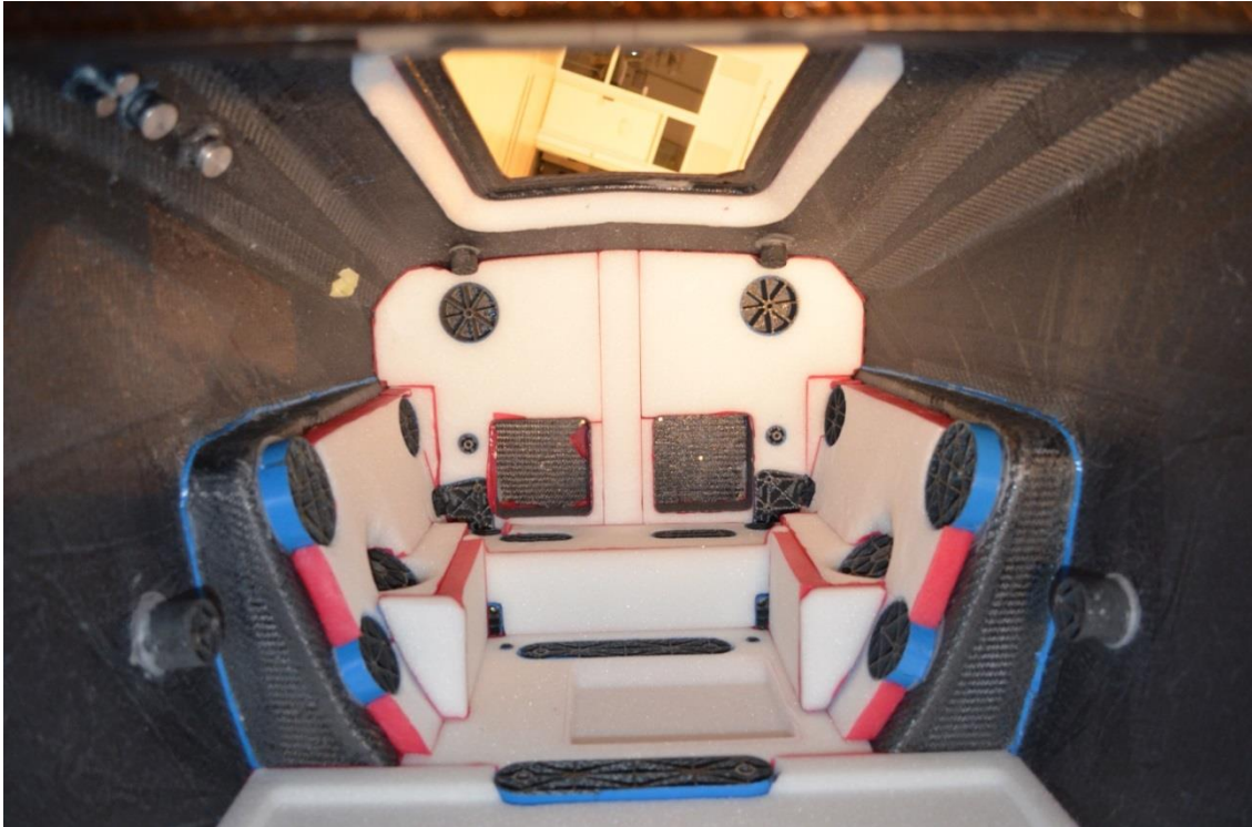
Figure 7.8: Placing of rohacell foam core in the rear end of the monocoque.
