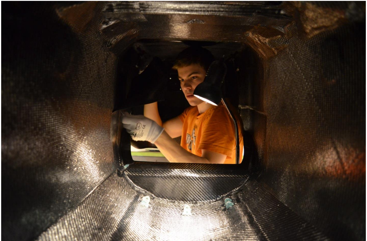
Figure 7.10: Layup of outer face sheet.
