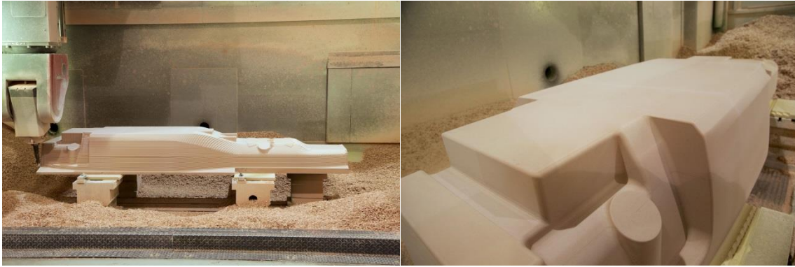
Figure 7.4: Machining of moulds
