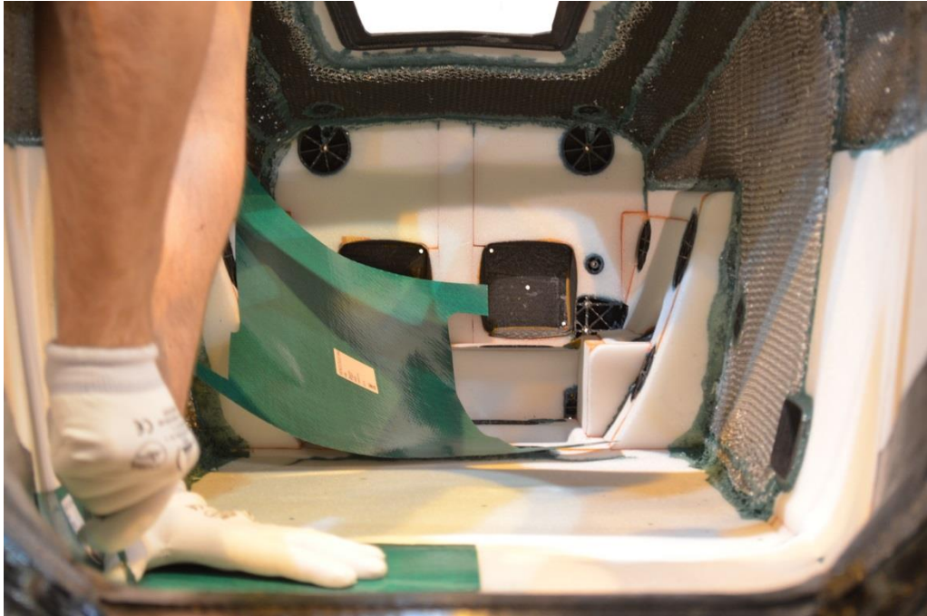
Figure 7.7: Layup of inner facesheet onto the core material.
