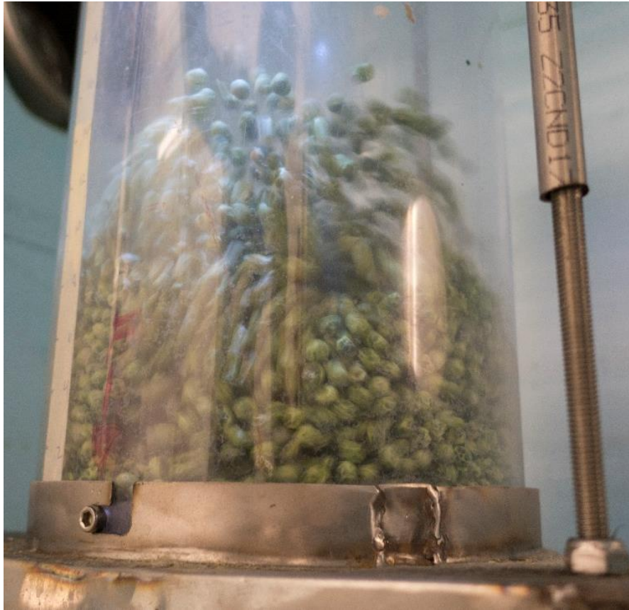
Figure 2: Gas fluidization Photo: Audun Rostad
