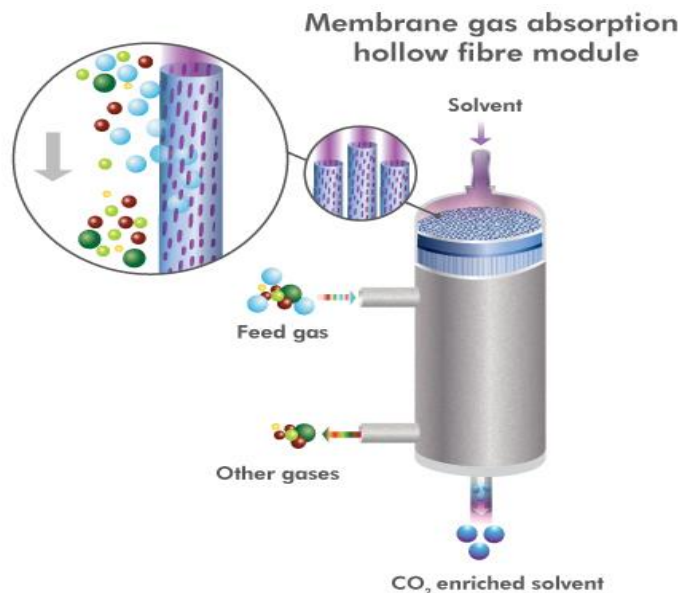
Figure 3-4: A Typical Hollow-fibre Membrane for CO 2 capture (CO 2 CRC, 2012)
