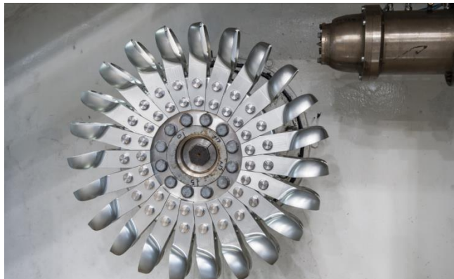
Figure 1 Pelton test rig at Waterpower Laboratory, NTNU (Buljo/NTNU, 2015)
