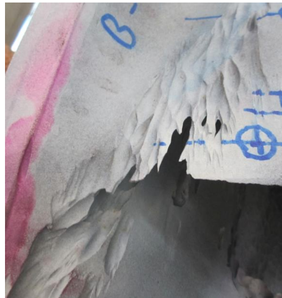
Figure 2 Eroded Francis turbine runner blade from Kaligandaki power plant (Writer's own photograph).
