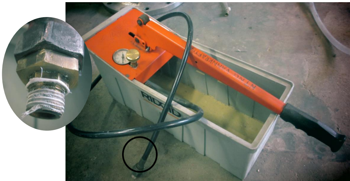
Figure 28 Manually operated water pump from Ridgid used at the Waterpower Laboratory (Writer's own image)
