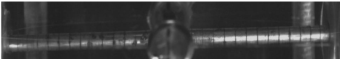
Figure 50 Calibration image used to measuring scale factor. The distance between each line is 5 mm (Writer's own image).
