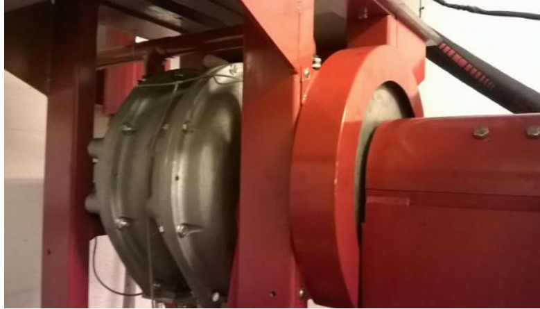
Figure 16: Hydraulic dynamometer (Water Brake) mounted to the engine.
