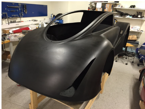
Figure 4.4: The monocoque with a smooth surface, before being foiled red
