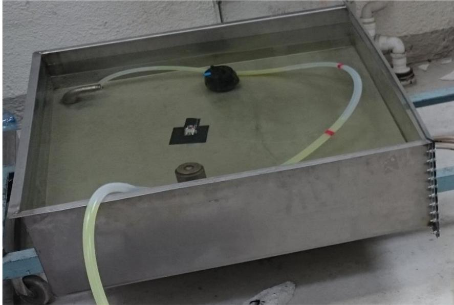
*Figure (3. 7): Tank used for DWH riser experiments (0.95 x 0.95 x 0.4 meters)*
