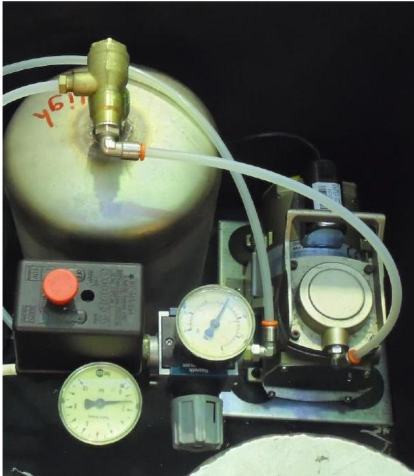
*Figure (3. 2): Compressor connected to high pressure tank*
