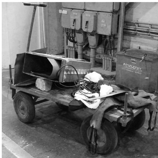
Figure 8.3: Mobile Faraday cage for transport of computer.
