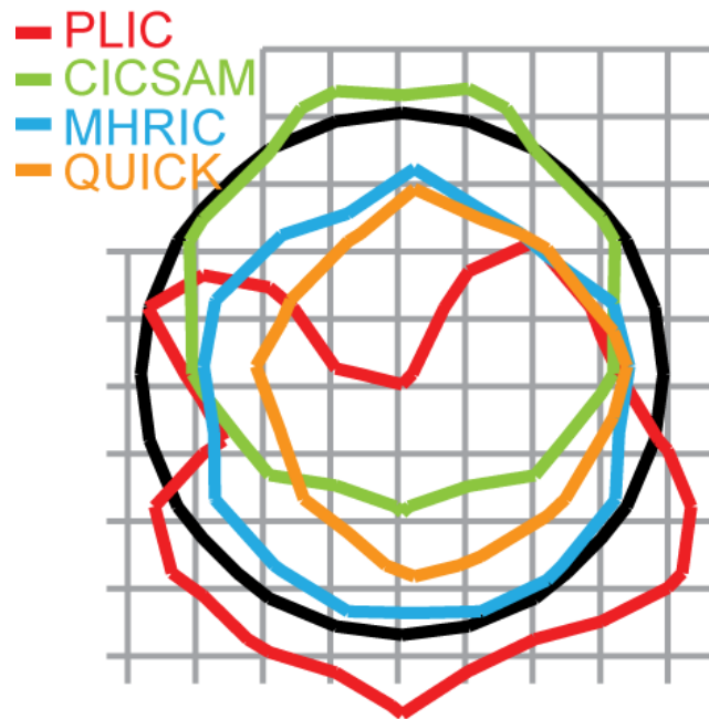
Figure A.5: 3D simulation of bubble on medium mesh ( a=40 ) using different discretization schemes for VOF, compared to the initial bubble surface (black).
