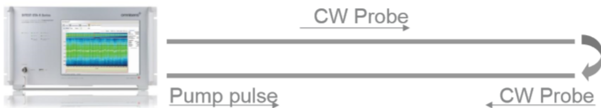
Figure 18: DTS monitoring unit based on SBS technology. [30]
