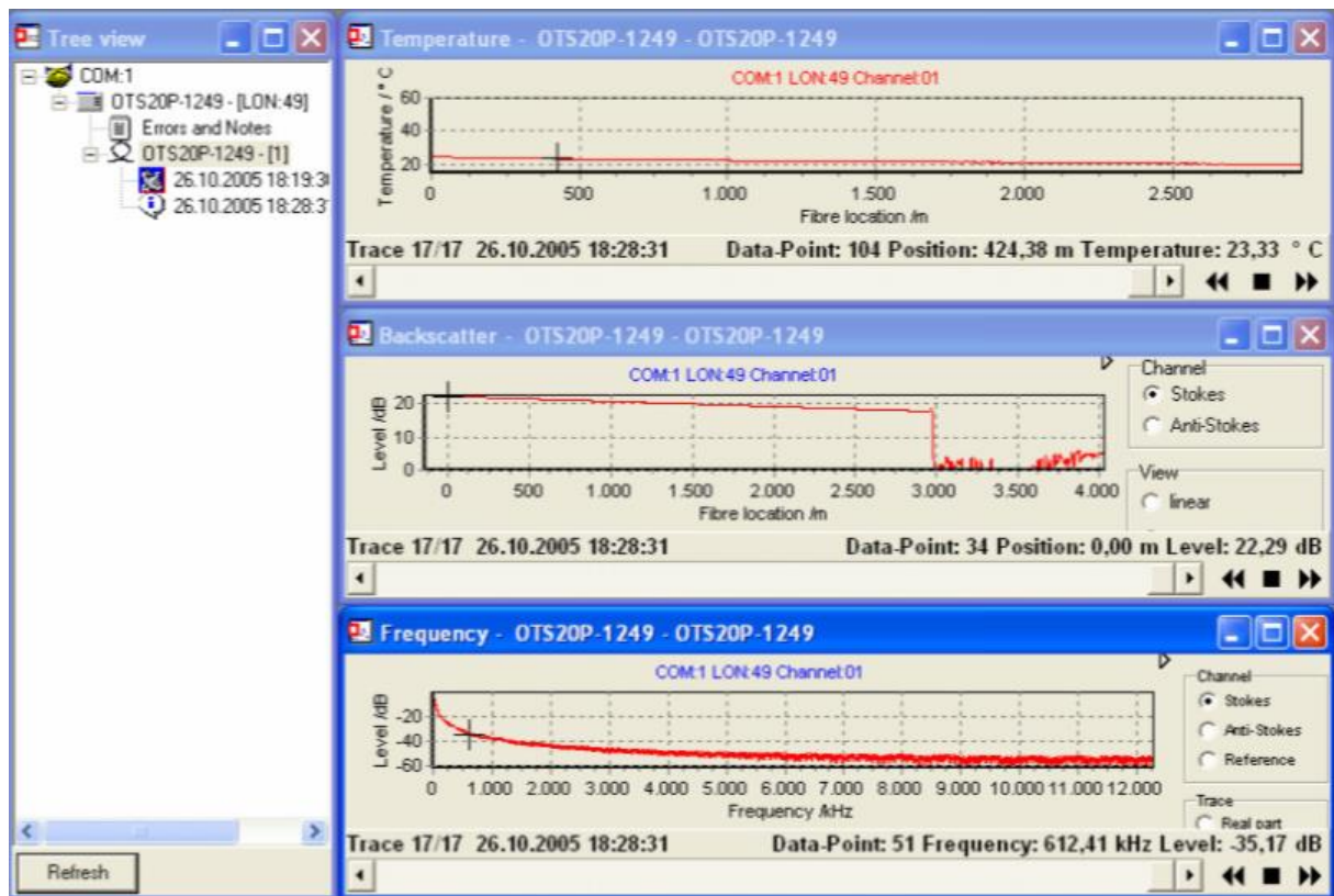
Figure 32: Frequency, backscatter and temperature profiles displayed in Charon_02. [29]
