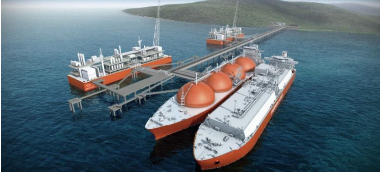
Figure 7: Principal sketch of the Höegh's near shore FLNG concept (Höegh LNG, 2015)
