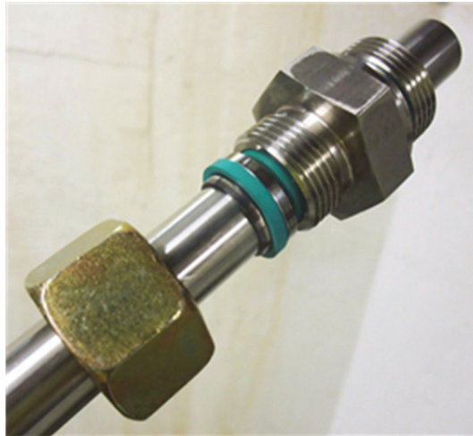
Figure 45 – Measurement probe with sealing system. Part with threads is mounted to the valve which is screwed on the pipe stub
