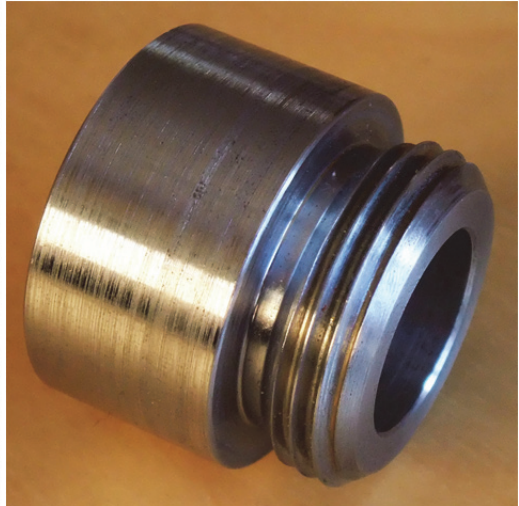
Figure 47 – Threaded pipe stub
