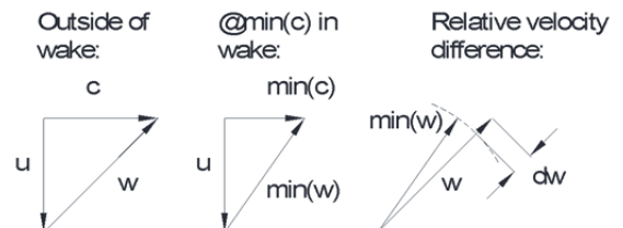
Figure 6 – Velocity diagram at rotor inlet
