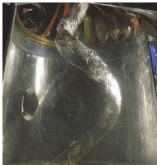
Figure 15 – Part load vortex rope [54]
