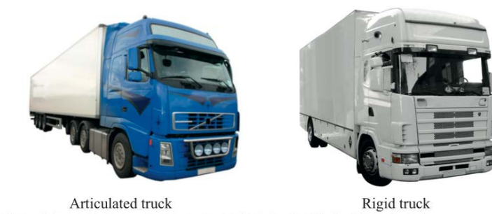
Figure 3: Articulated truck (to the left) and rigid truck (to the right) (Levin, 2012).
