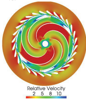
Figure 14 Iso-plot of relative velocity in operation point 4
