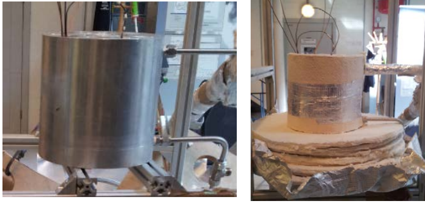
Figure 5.4: Placement of heat storage on the oil rig without insulation (left) and with parts of the insulation applied (right)
