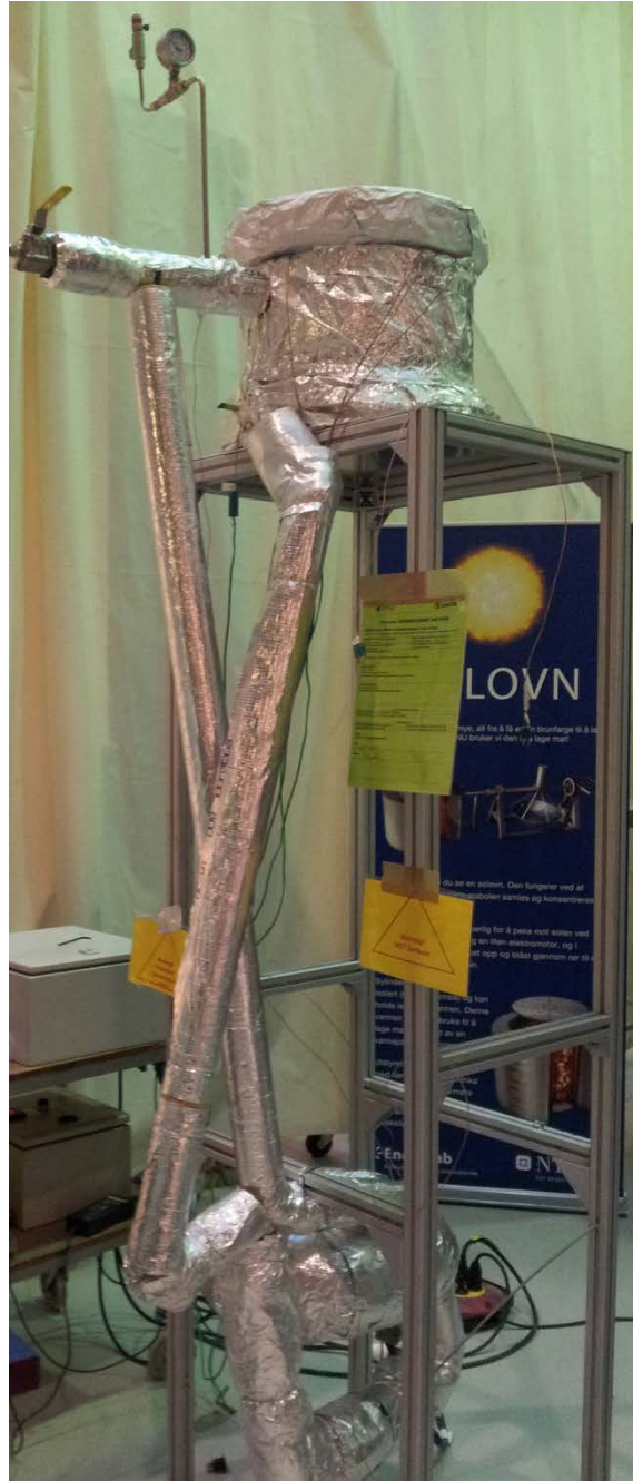
Figure 5.9: Set up of the storage and steam system during Experiment 2
