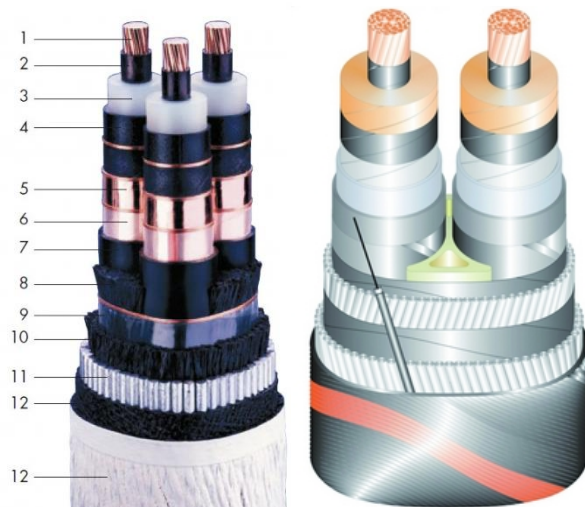
Figure 17: Cable compositions. Left: XLPE three-core 36 kV AC cable [37]. Right: the NorNed flat mass-impregnated HVDC cable [25]. Except for the insulation, the materials are more or less the same.
