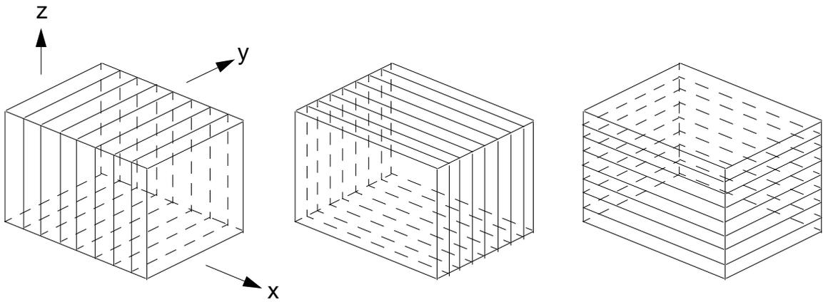
The partitioning process itself is partially controllable through the direction specification. However, in general, larger overlap regions occur compared with both the MeTiS and recursive coordinate bisection partitioners.
