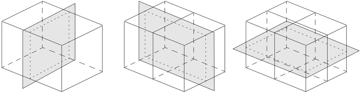
Like MeTiS, the Recursive Coordinate Bisection partitioner uses a fast, fully automatic algorithm, but it has only a small additional memory overhead. A particular disadvantage is that larger overlap regions can exist compared with the MeTiS partitioner, and each partition may contain separate parts.
