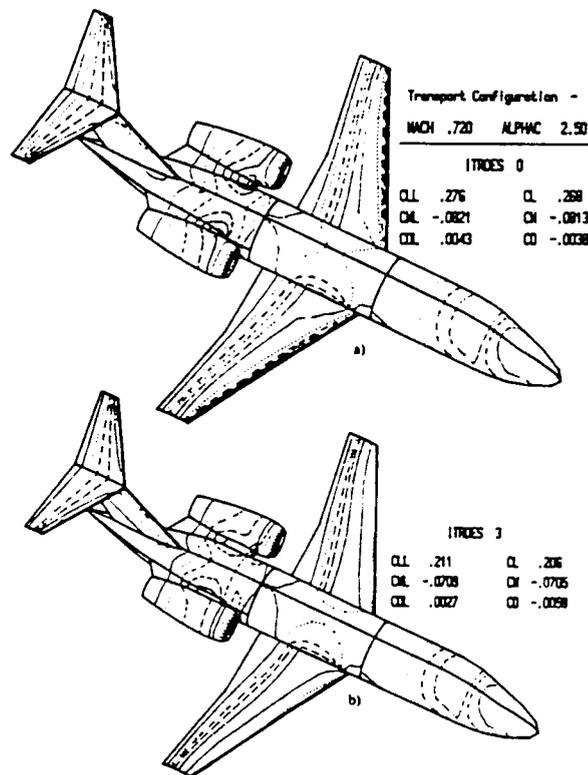
Fig. 6 Entire business jet configuration can be optimized<sup>53</sup> on a personal computer using surface transpiration concept and a panel method a) before and b) after three optimization cycles. Notice improvements in aerodynamic coefficients.
