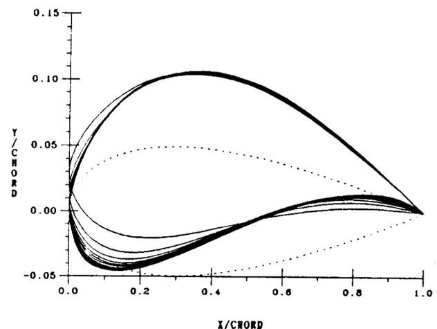
Fig. 2 Example of the convergence history using a master code method<sup>24</sup> and a surface panel analysis code; initial shape was a NACA0010 airfoil; and target pressure distribution was for a 15%-thick cambered Zhukovskii airfoil.
