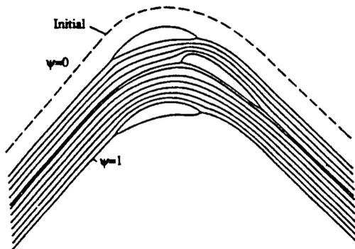
Fig. 3 SFC method<sup>36</sup> generates streamline shapes directly as its solution; example of a turbomachinery cascade designed simultaneously with a splitter blade in a single computer run.
