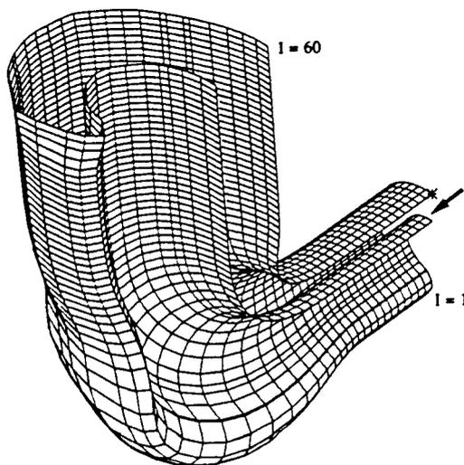
Fig. 4 Stream function—potential function inverse design method,<sup>30</sup> can generate complex realistic three-dimensional configurations.
