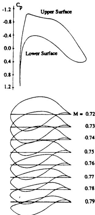
Fig. 1 Airfoil shapes<sup>15</sup> ( $y$ -axis magnified five times) having identical surface pressure distributions at different freestream Mach numbers.
