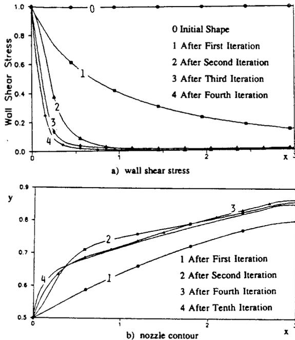
Fig. 7 Two-dimensional nozzle designed using laminar incompressible Navier-Stokes equations and adjoint operator/control theory<sup>77-79</sup>; iteration histories for a) the surface shear stress and b) the nozzle geometry. Inlet-to-exit pressure rise was maximized while minimizing total pressure loss.
