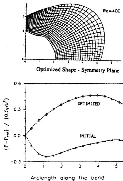
Fig. 8 Three-dimensional curved duct designed using Navier-Stokes equations and adjoint operator/control theory<sup>80</sup>; initial duct had constant radius; and inlet-to-exit pressure rise was maximized while minimizing total pressure loss.
