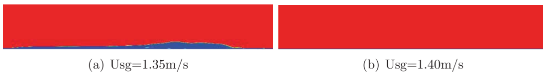
Figure 2.12: LL=0.1\% . The situation for the Low Mesh when no friction dominated solution was found. Blue is liquid, red is gas. Only a section illustrated.
