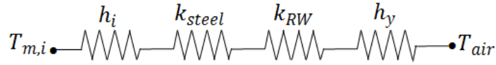
Figure 4.8: Resistance network for the heat transfer from the inside of the tube to the surroundings.
