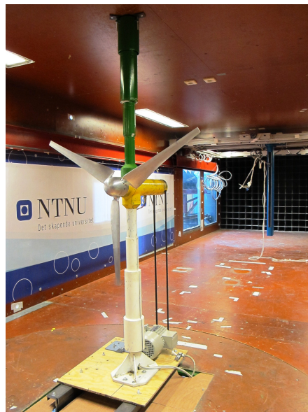
Figure 3.10: Turbine with additional tower
