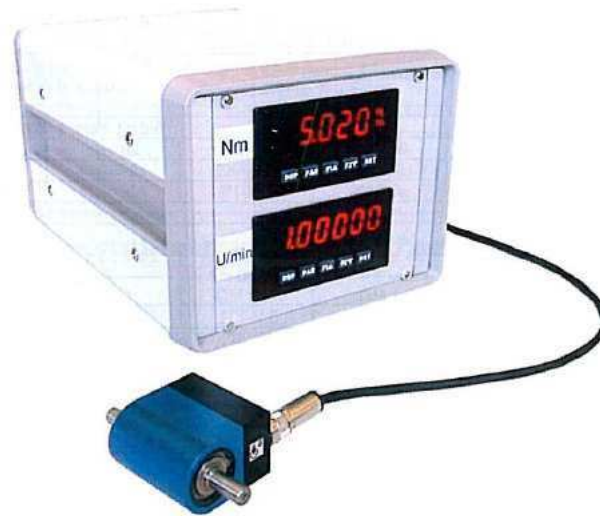
Figure 3.4: Torque meter and rotation speed sensor with digital display [20]
