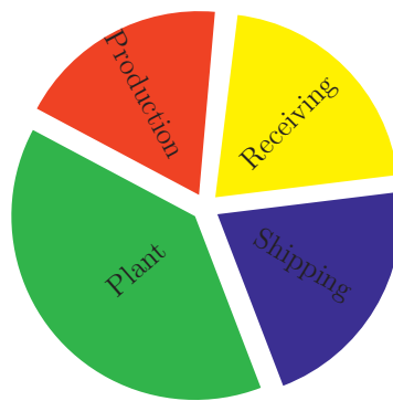
Figure 1.2: Division of costs in GTL value chain. Production : gas production, from the reservoir to the LNG plant (15 – 20%); Plant : LNG plant, gas treating, liquefaction, LPG and condensate recovery (30 – 45%); Shipping : transport to final destination (10 – 30%); Receiving : unloading, storage, re-gasification and distribution (15 – 25%)
