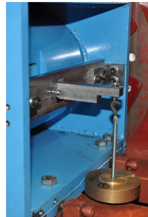
(f) Lever arm and weight for calibrating.
