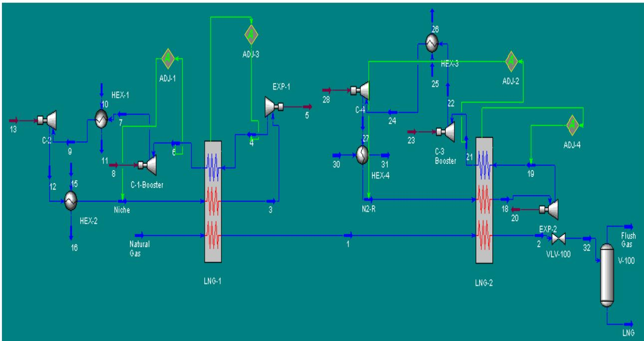
**Figure 45:** Process flow diagram for Niche LNG Process
