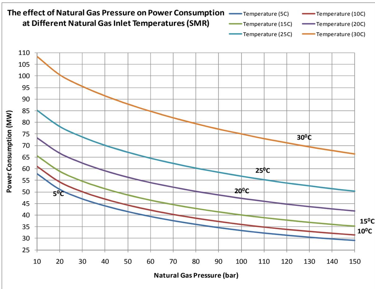
**Figure 19:** The effect of Natural gas pressure on power consumption when natural gas supplied at different temperatures (SMR-PRICO)
