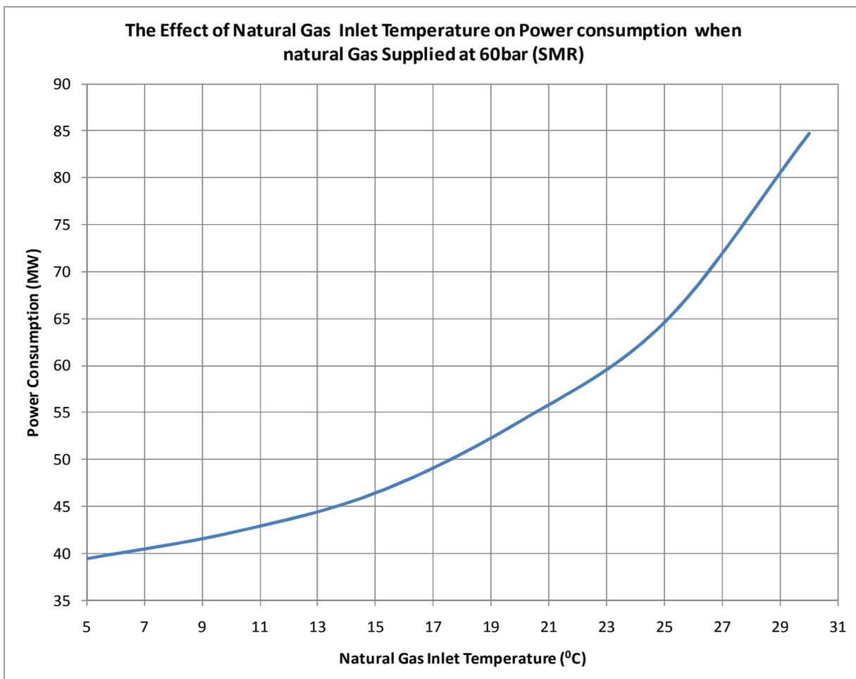
**Figure 12:** The effect of natural gas supply temperature on power consumption when natural gas supplied at 60ba (SMR PRICO)
