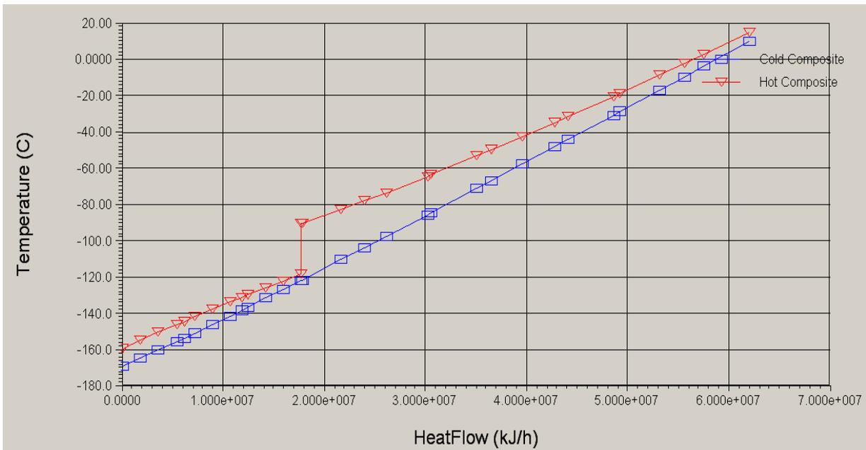
Composite curve for LNG heat exchanger LNG-1 (Niche LNG process)
