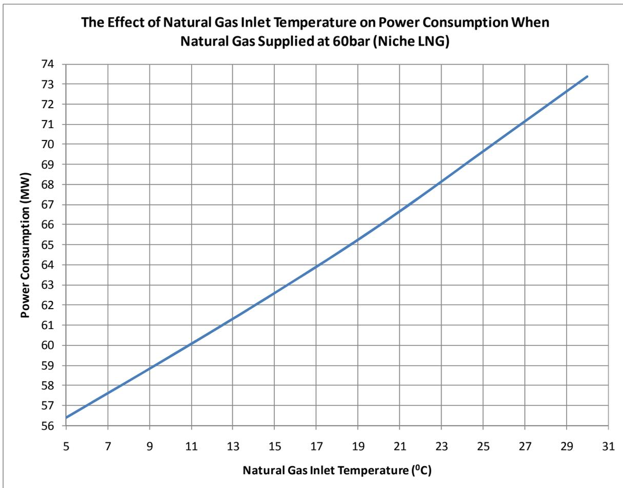
**Figure 48:** The effect of natural gas inlet temperature of power consumption when natural gas supplied at 60bar (Niche LNG)
