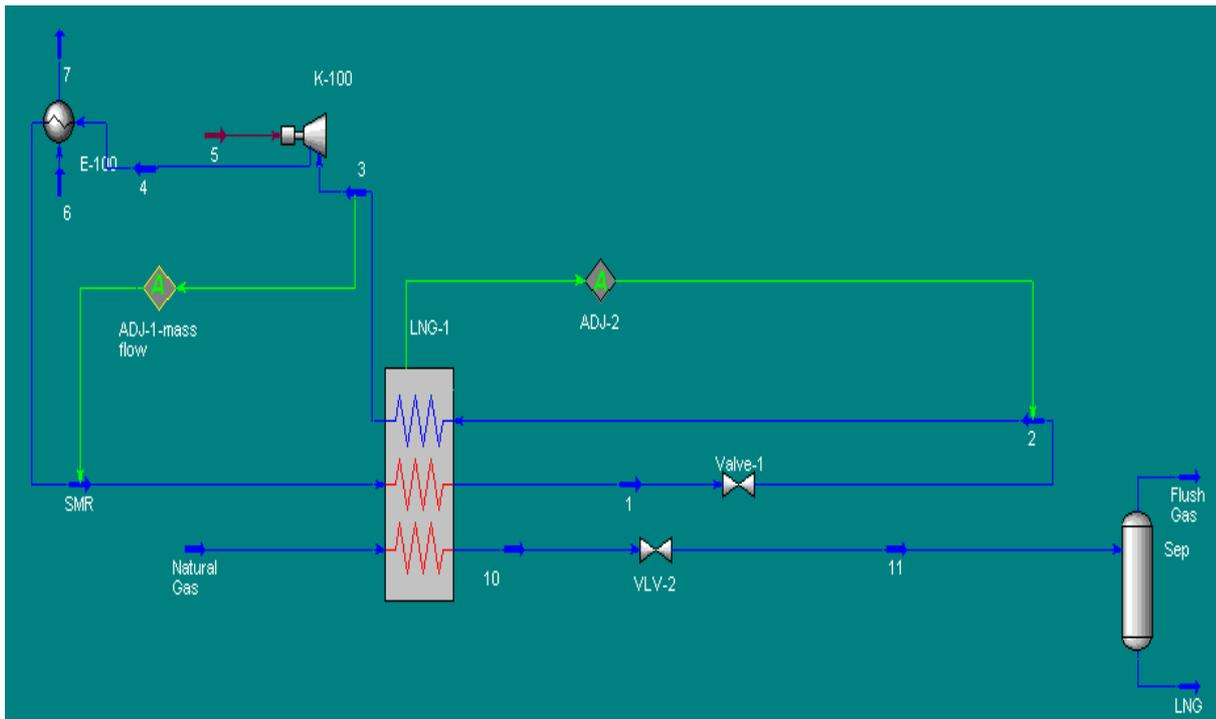
**Figure 9:** Process Flow Diagram of SMR (PRICO)
