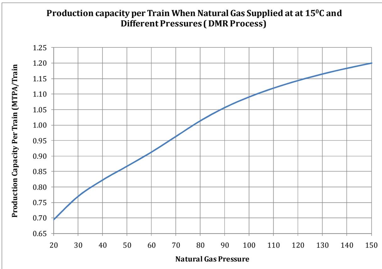
**Figure 44:** The production capacity of DMR
