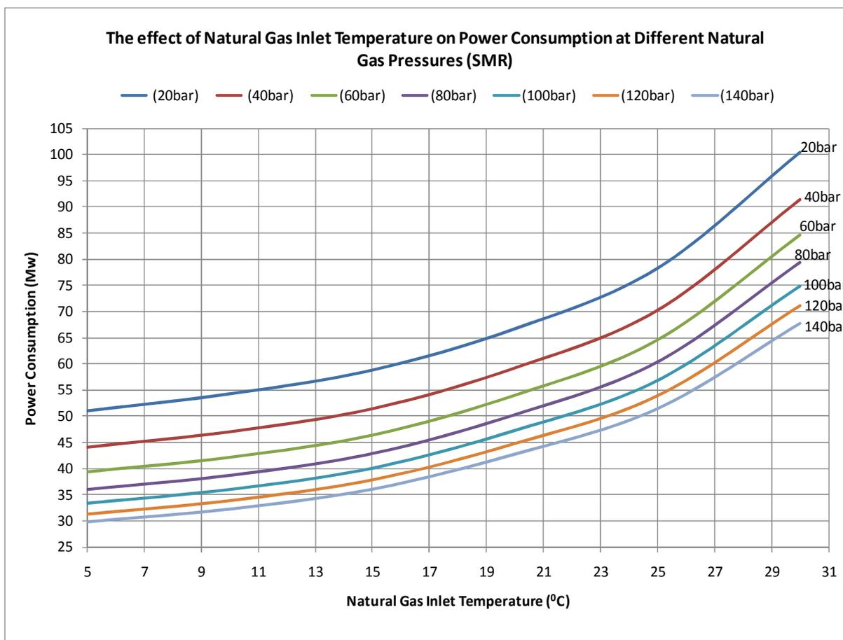
**Figure 13:** The effect of natural gas inlet temperature on power consumption at different Pressures (SMR PRICO)
