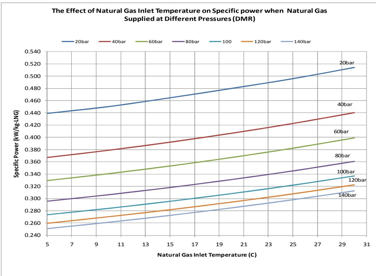
**Figure 29:** The effect of natural gas inlet temperature on specific power when natural gas supplied at different pressures (DMR Process)
