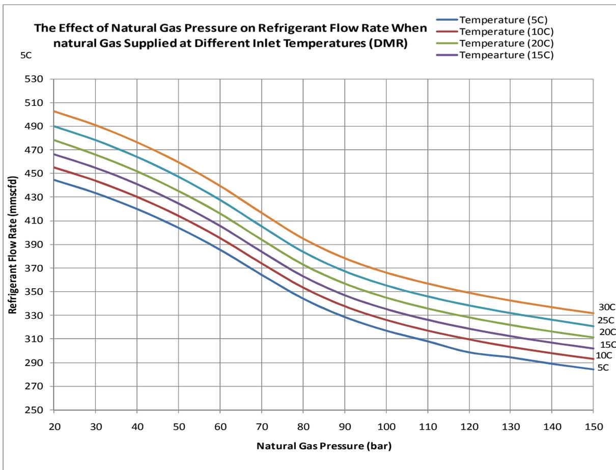
**Figure 39:** The effect of natural gas pressure on refrigerant flow when natural gas supplied at different temperatures (DMR).
