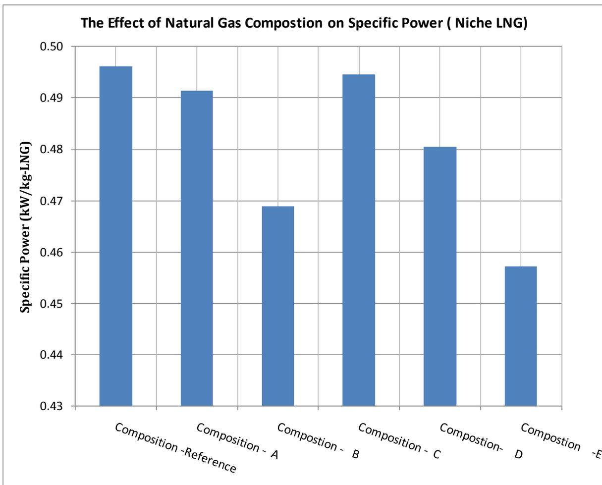
**Figure 54:** The effect of natural gas composition on specific power (Niche LNG)
