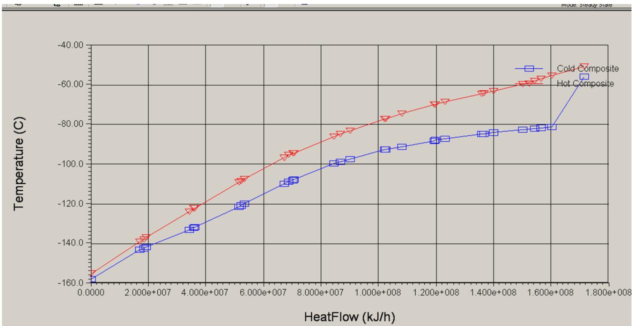
Composite curve for LNG heat exchanger LNG-2 (DMR process)
