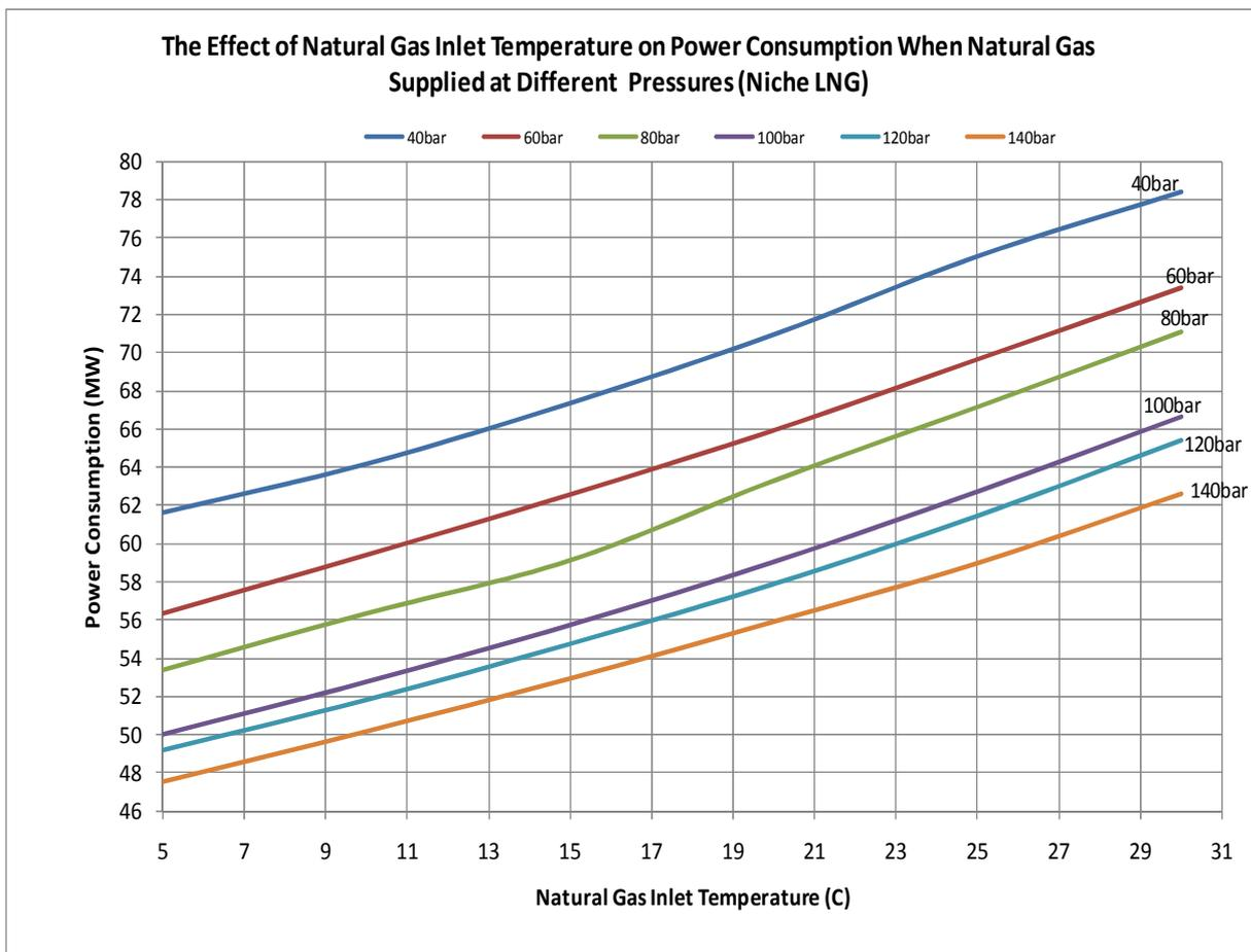
**Figure 49:** The effect of natural gas inlet temperature on power consumption when natural gas supplied at different temperatures (Niche LNG)
