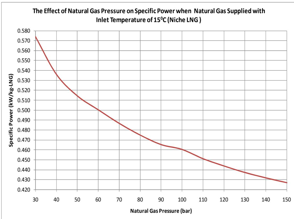
**Figure 50:** The effect of natural gas pressure on specific power when natural gas supplied with inlet temperature of 15°C (Niche LNG Process)
