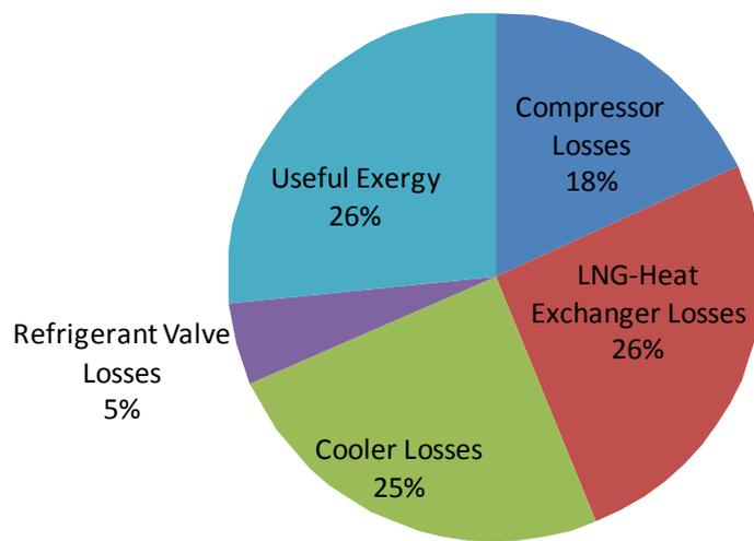
**Figure 25:** Distribution of Exergy losses on different components and useful exergy (SMR PRICO)
