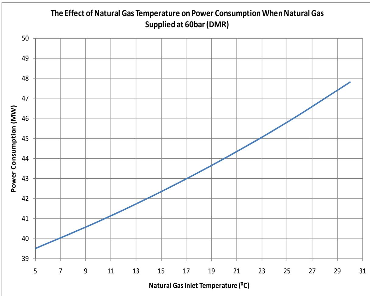
**Figure 30 :** The effect of natural gas temperature on power consumption when natural gas supplied at 60bar (DMR Process)
