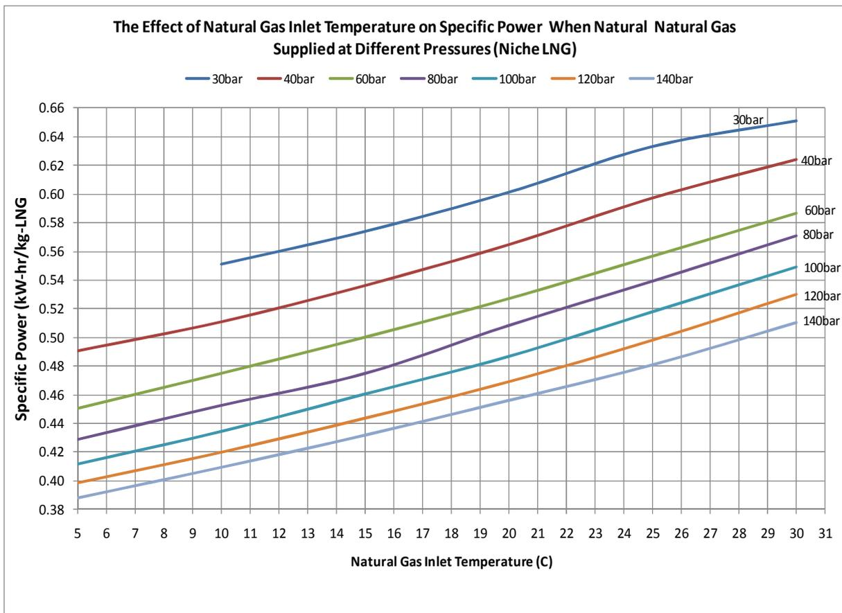
**Figure 47:** The effect of natural gas temperature on specific power when natural gas supplied at different pressures (Niche LNG Process)
