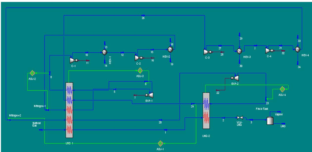
**Figure 59** : Process flow diagram of dual nitrogen expander process
