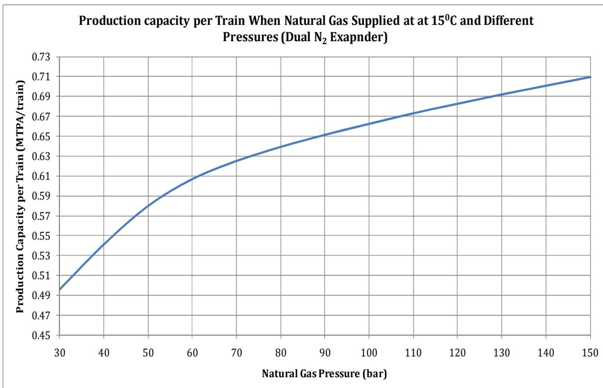
**Figure 72:** Production capacity per train when natural gas supplied at 15°C and Different pressure (Dual Nitrogen Expander)
