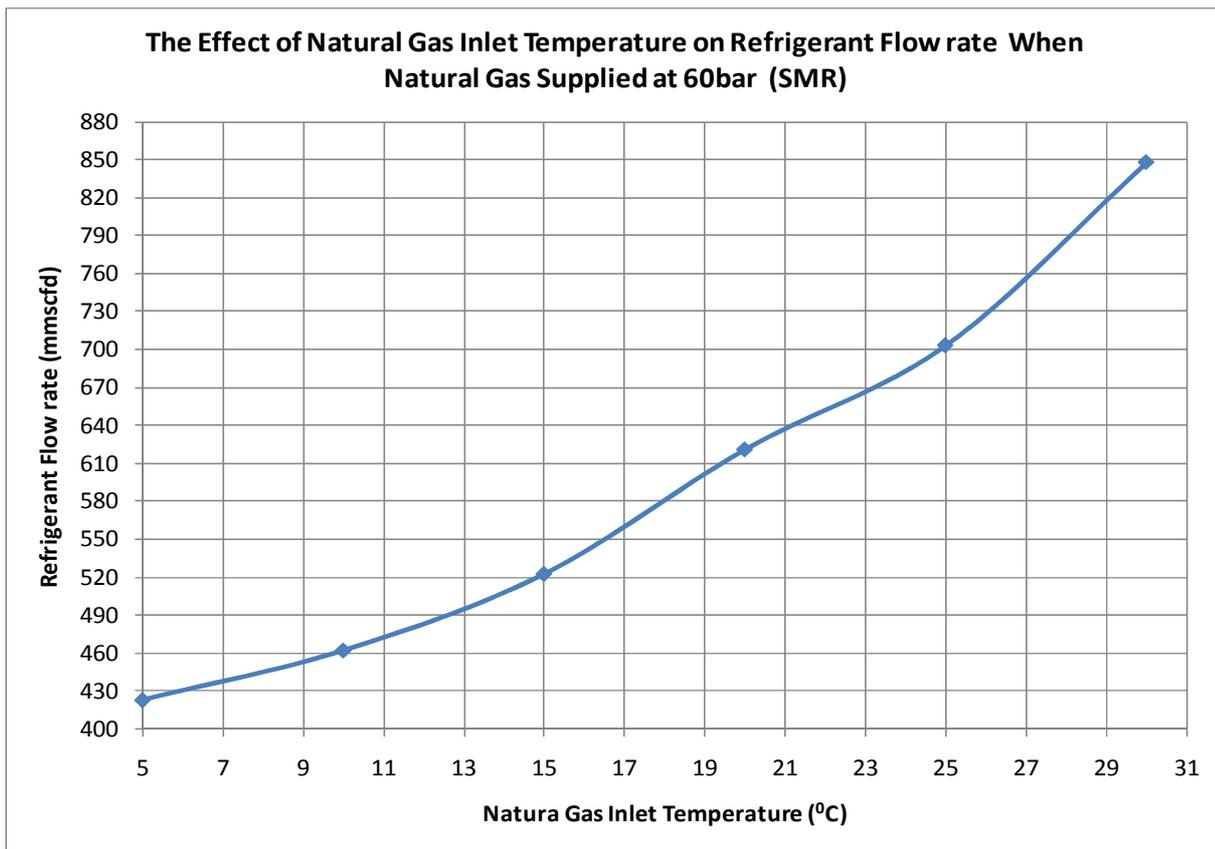
**Figure 14 :** The effect of natural gas inlet temperature on refrigerant flow rate when natural gas supplied at 60 bar (SMR PRICO)
