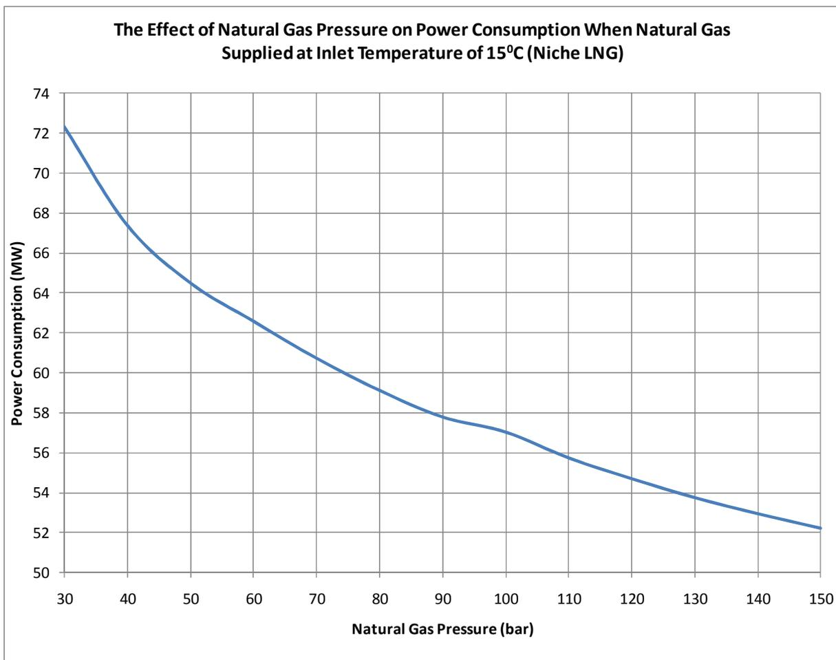
**Figure 52 :** The effect of natural gas pressure on power consumption when natural gas supplied at inlet temperature of 15°C (Niche LNG Process).
