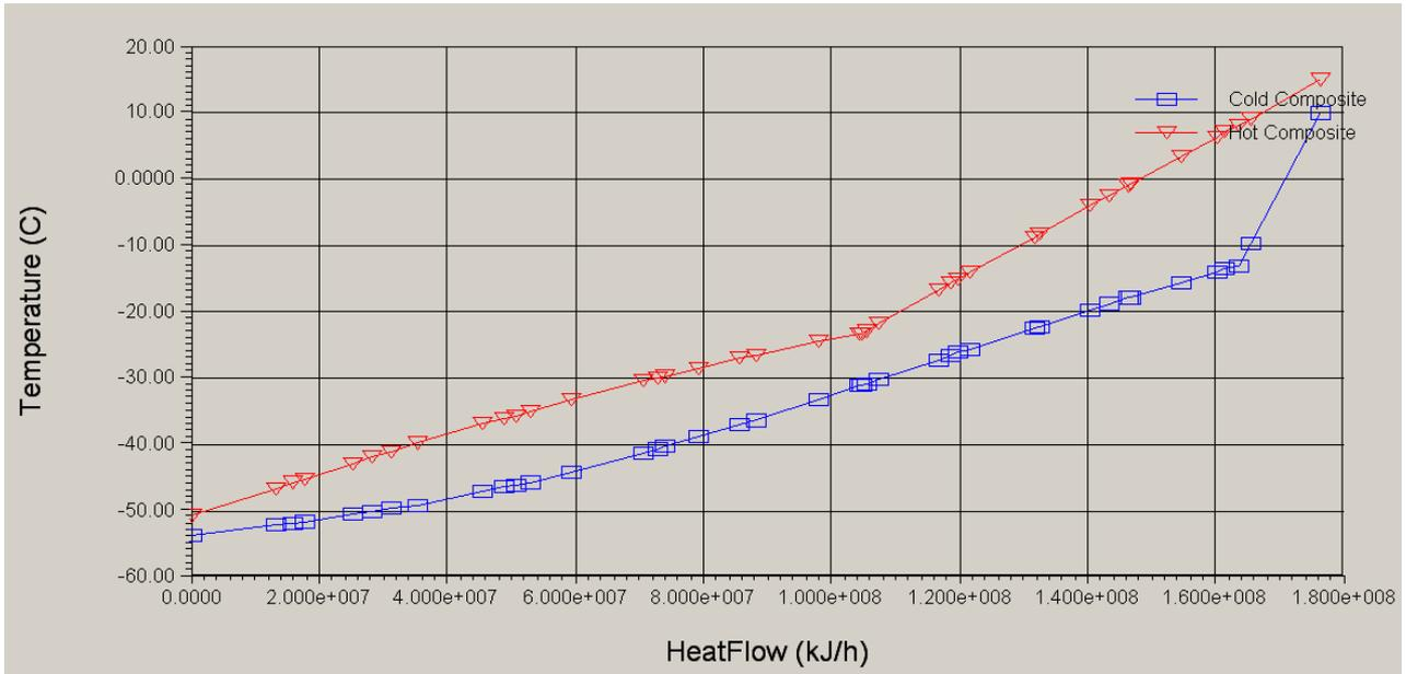
Composite curve for LNG heat exchanger LNG-1 (DMR process)
