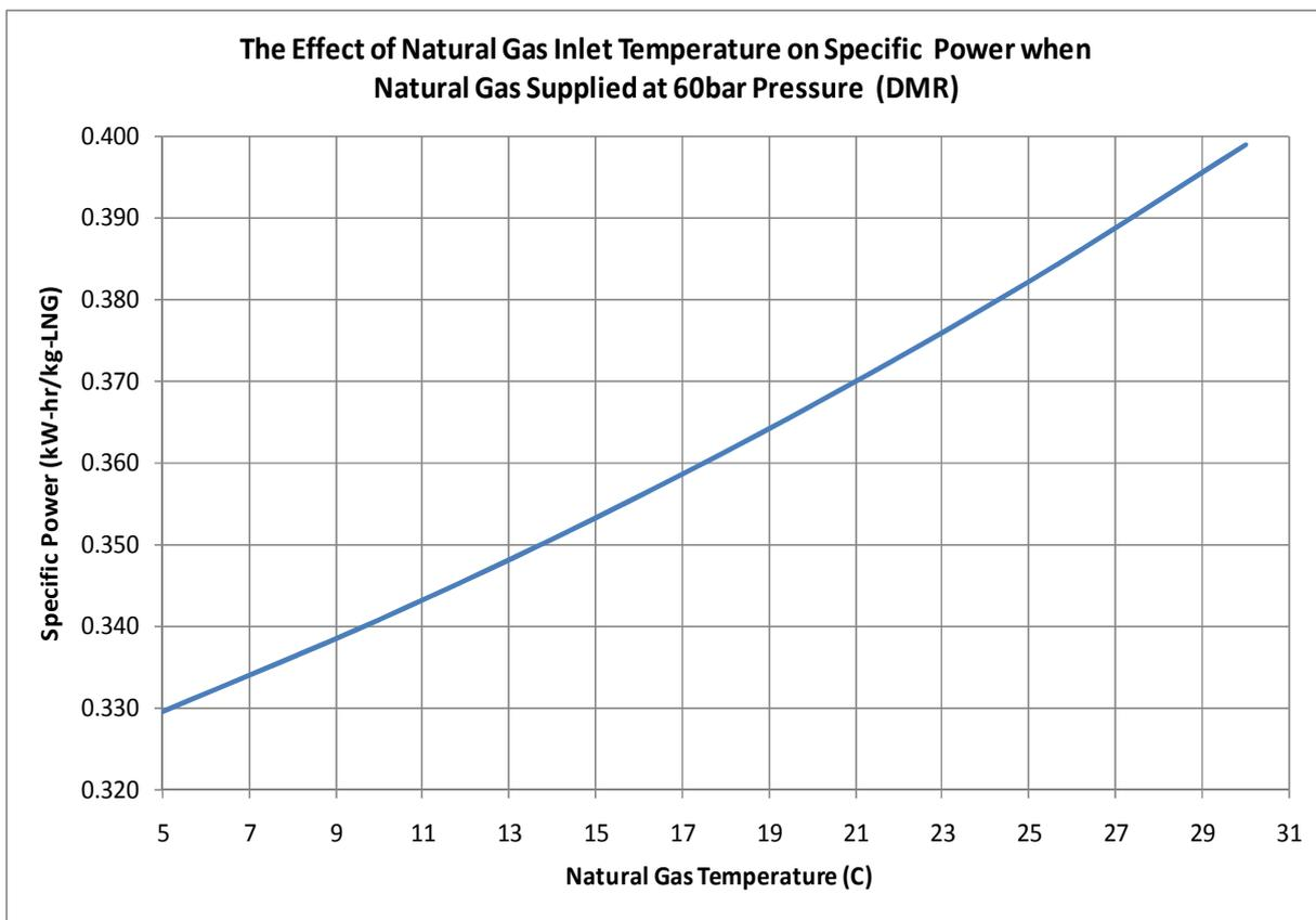
**Figure 28:** The effect of natural gas temperature on specific power when natural gas supplied at 60bar (DMR Process)
