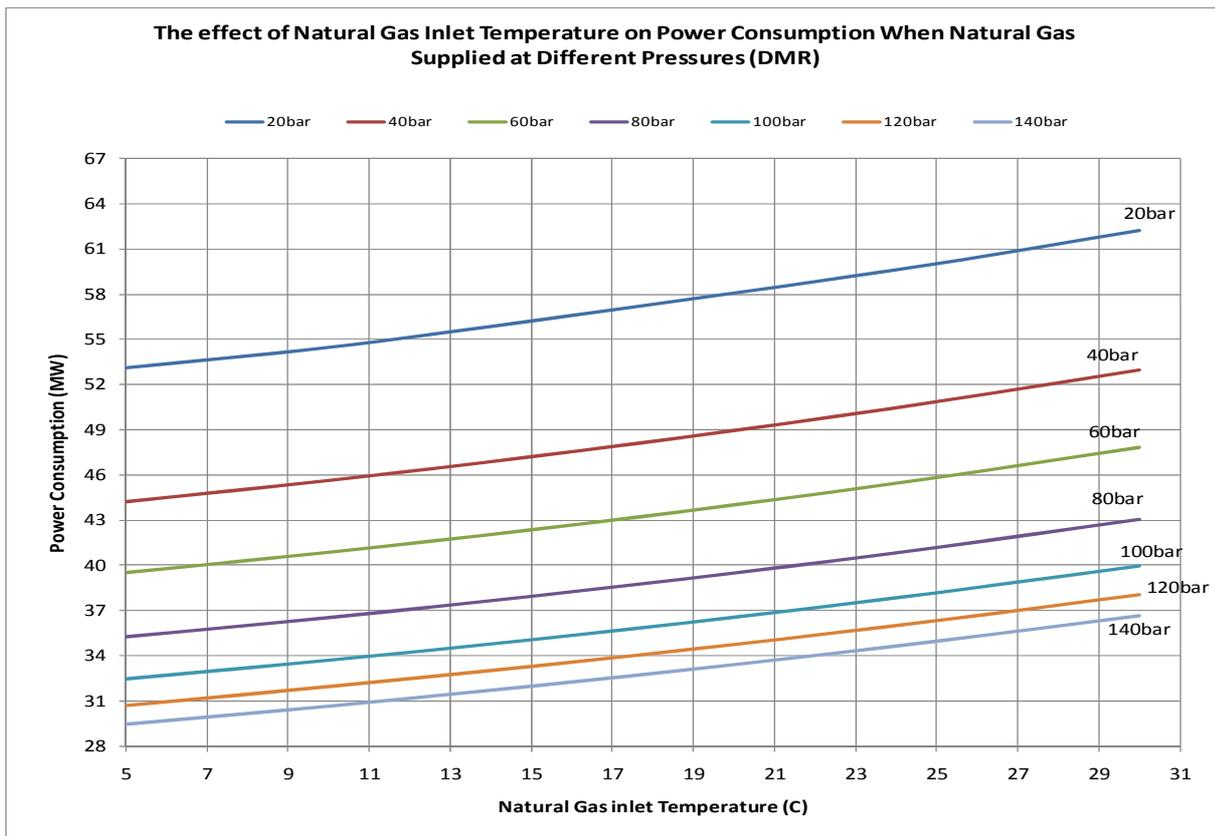
**Figure 31:** The effect of natural gas temperature on power consumption when natural gas supplied at different temperatures (DMR Process).
