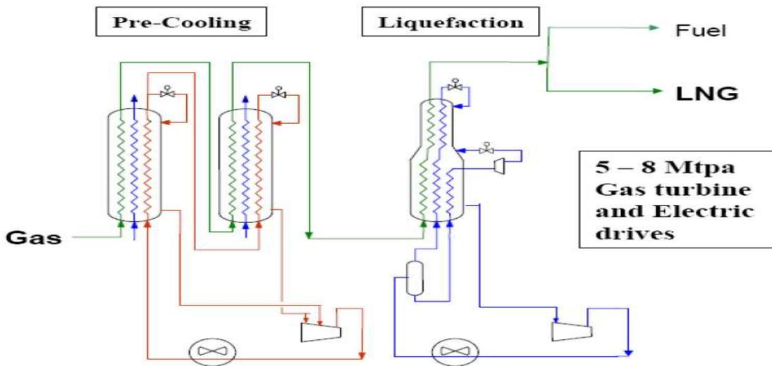
**Figure 7:** Diagram of dual mixed refrigerant process (Source [16])
