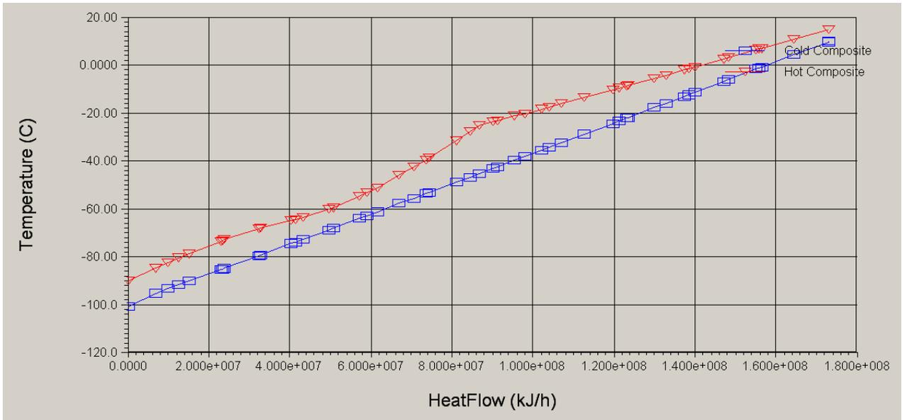
Composite curve for LNG heat exchanger LNG-1 (dual nitrogen expander process)
