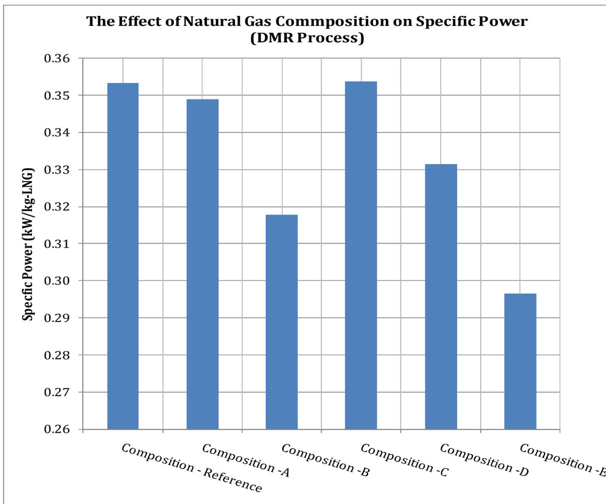
**Figure 40:** The effect of natural gas composition on specific power (DMR Process)
