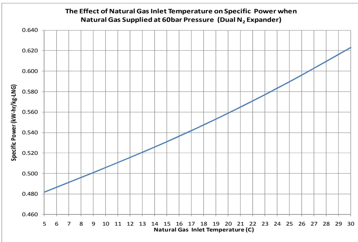
**Figure 60:** The effect of natural gas inlet temperature on specific power when natural gas supplied at 60bar (Dual N<sub>2</sub> Expander Process).
