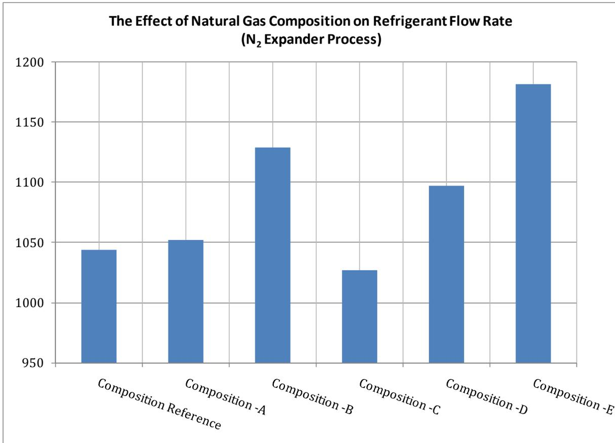
**Figure 70:** The effect of natural gas composition on refrigerant flow rate dual N<sub>2</sub> expander process
