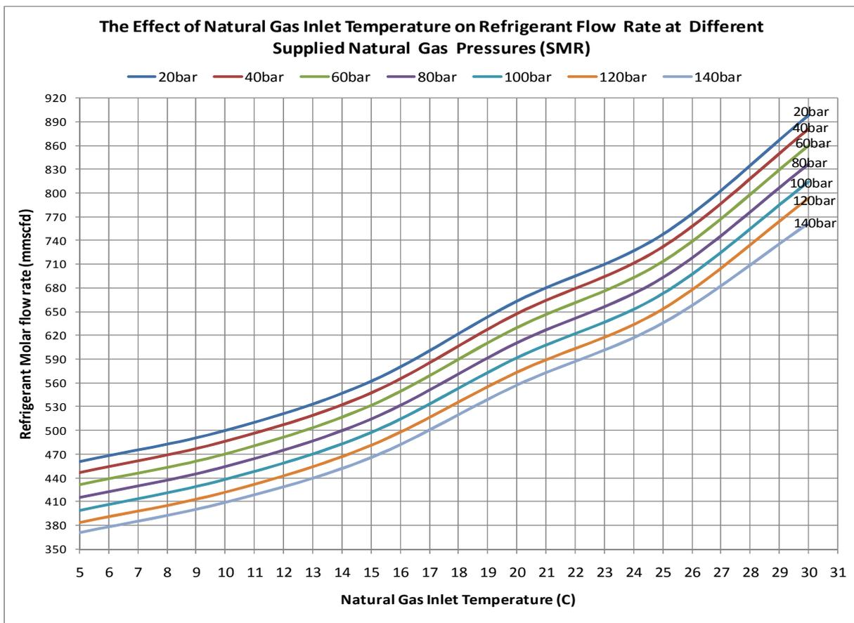
**Figure 15:** The effect of natural gas inlet temperature on refrigerant flow rate at different natural gas supplied pressures (SMR- Process)
