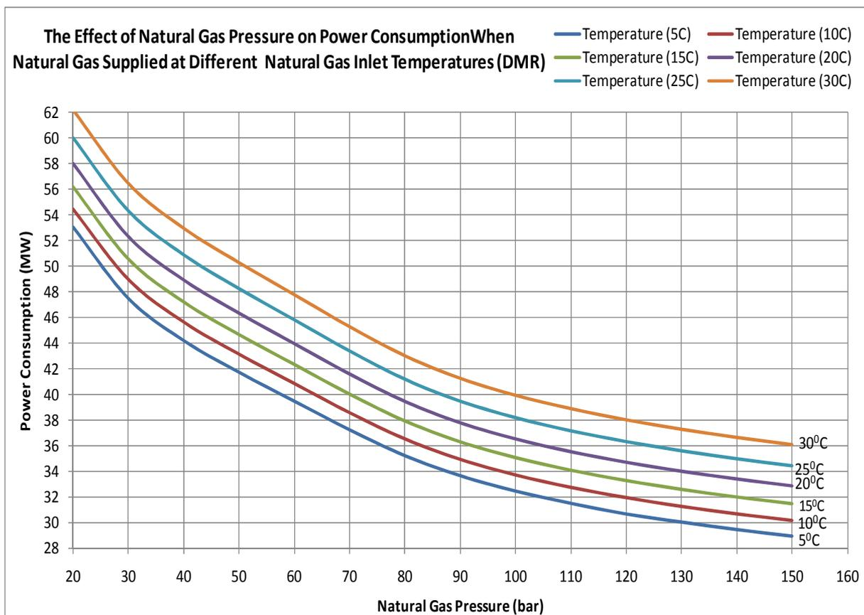
**Figure 37:** The effect of natural gas pressure on power consumption when natural gas supplied supplied at different temperature (DMR Process)
