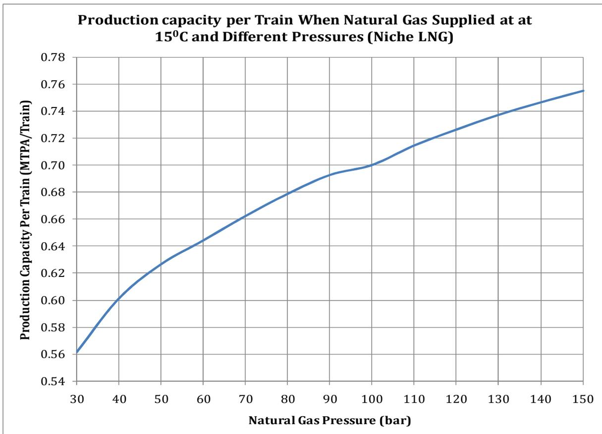
**Figure 58:** The production capacity of Niche LNG Process
