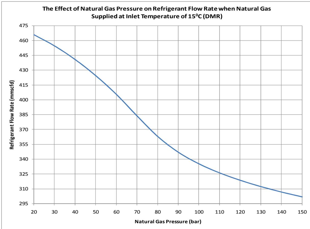
**Figure 38:** The effect of natural gas pressure on refrigerant flow rate when natural gas supplied at inlet pressure of 15°C (DMR Process)
