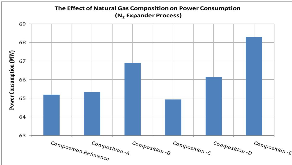
**Figure 69:** The effect of natural gas composition on power consumption dual N<sub>2</sub> expander Process
