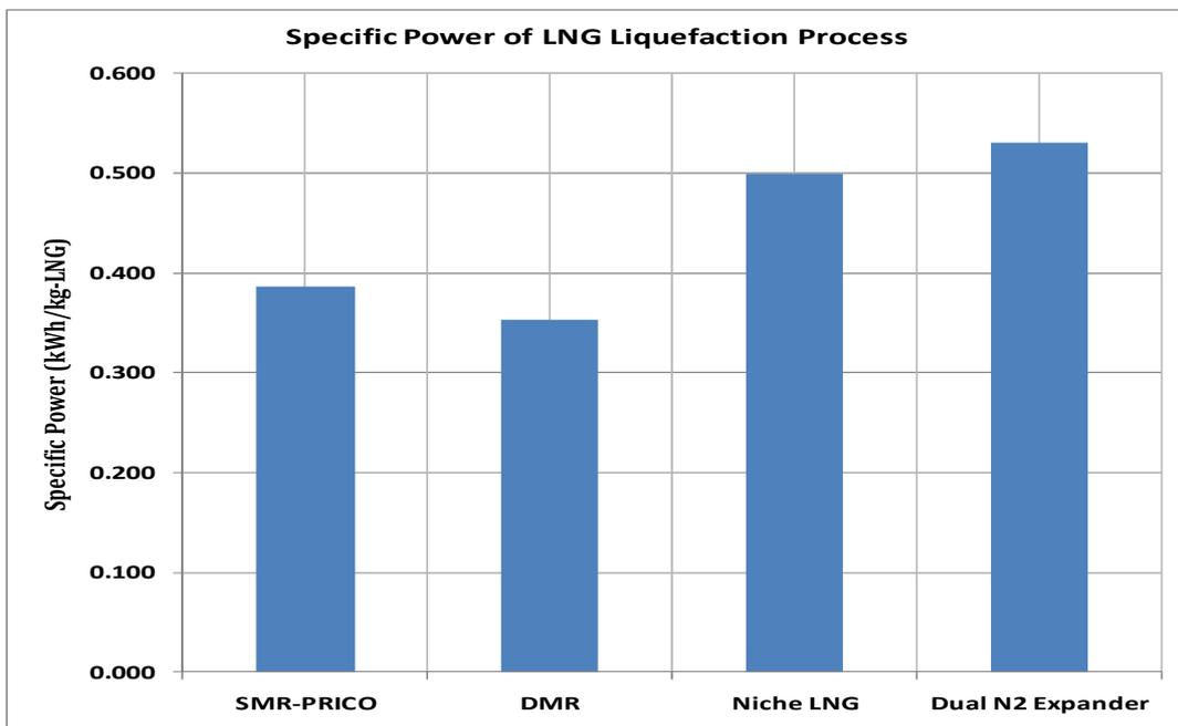
**Figure 73** : The comparison of the specific power of proposed liquefaction processes for LNG FPSO
