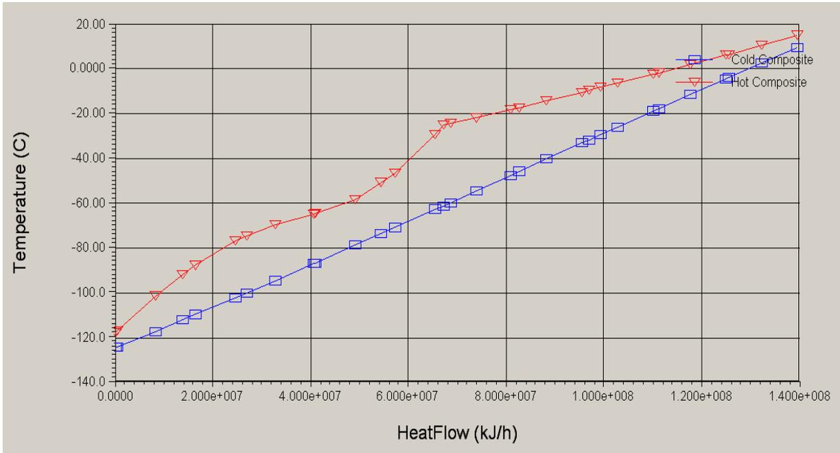
Composite curve for LNG heat exchanger LNG-1 (Niche LNG process)
