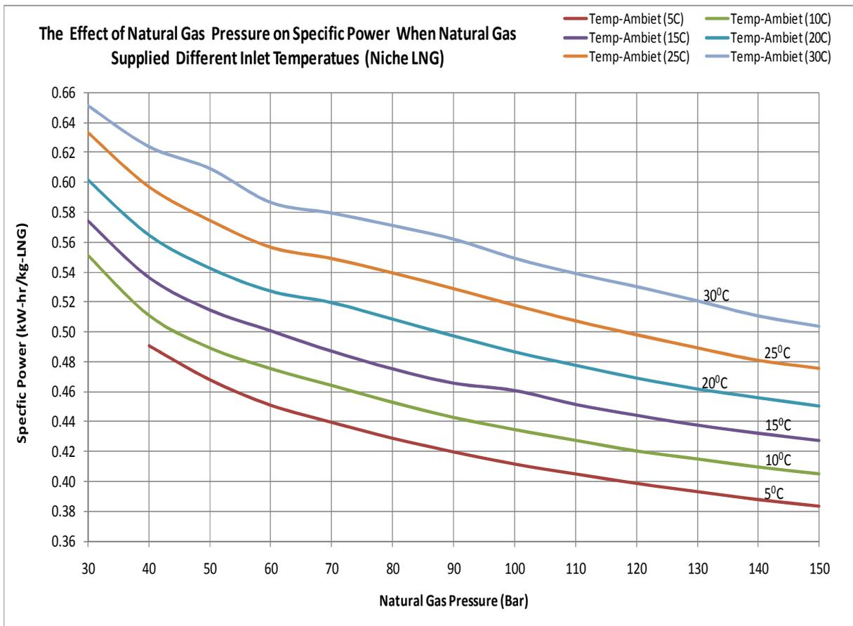
**Figure 51:** The effect of natural gas pressure on specific power when natural gas supplied at different temperature (Niche LNG Process)
