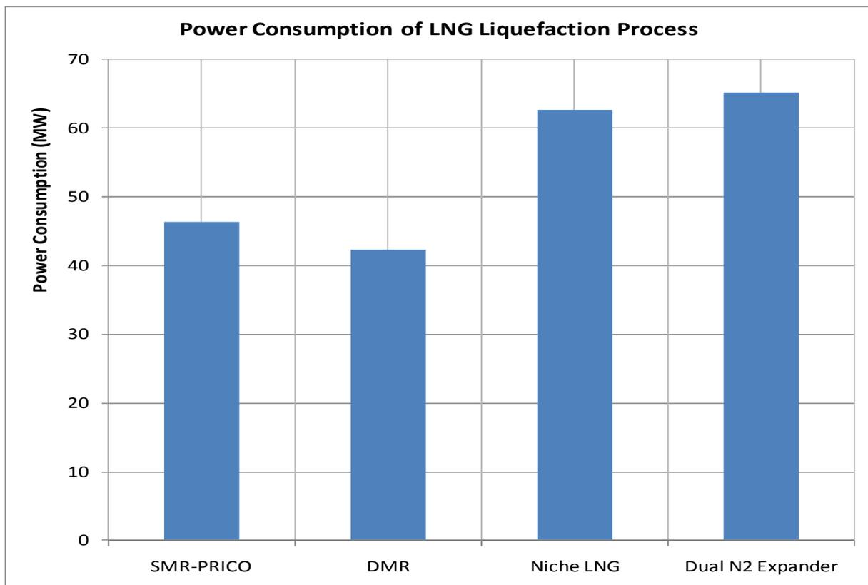
**Figure 74:** Comparison of power consumption of the proposed liquefaction processes for LNG FPSO
