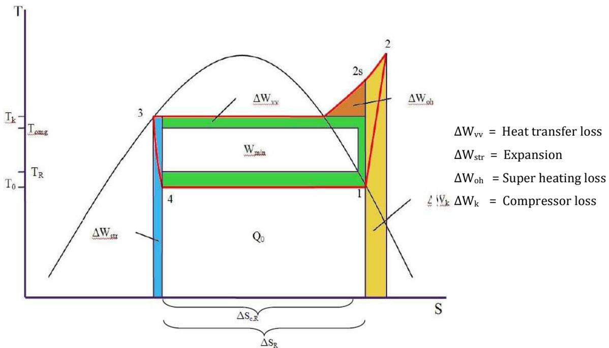
**Figure 5:** Temperature/entropy diagram showing different losses in refrigeration cycle
