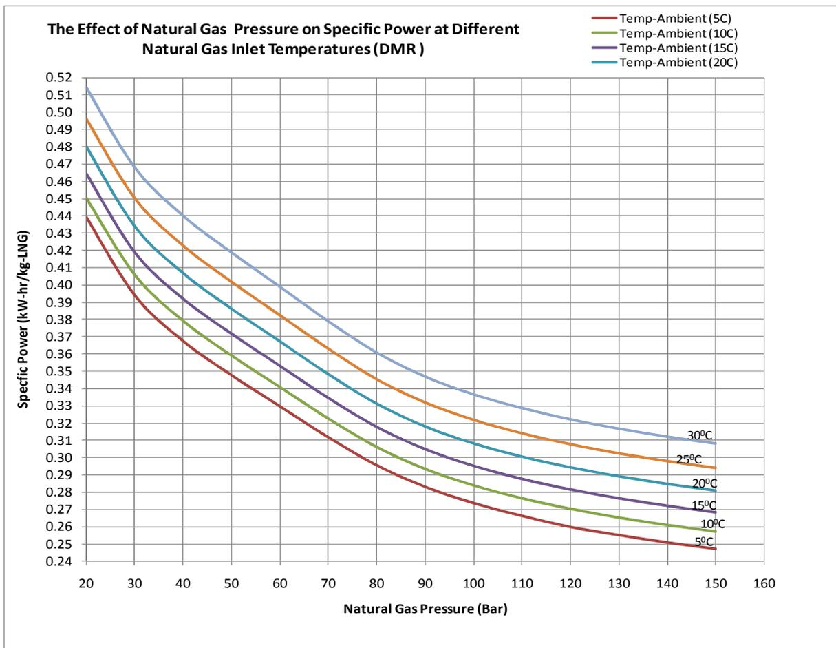
**Figure 35 :** The effect of natural gas pressure on specific power when natural gas supplied at different temperatures (DMR Process)
