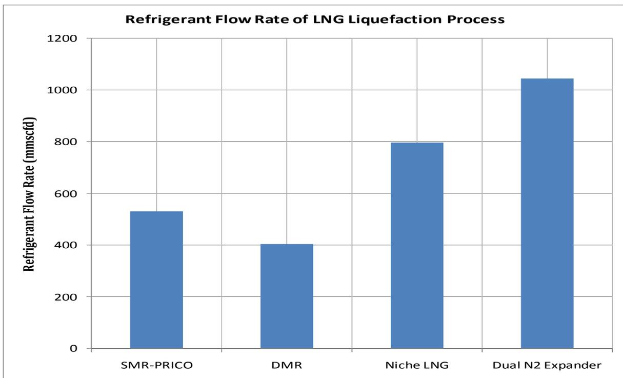
**Figure 75:** The comparison of refrigerant flow rate of the proposed LNG liquefaction process for LNG FPSO
