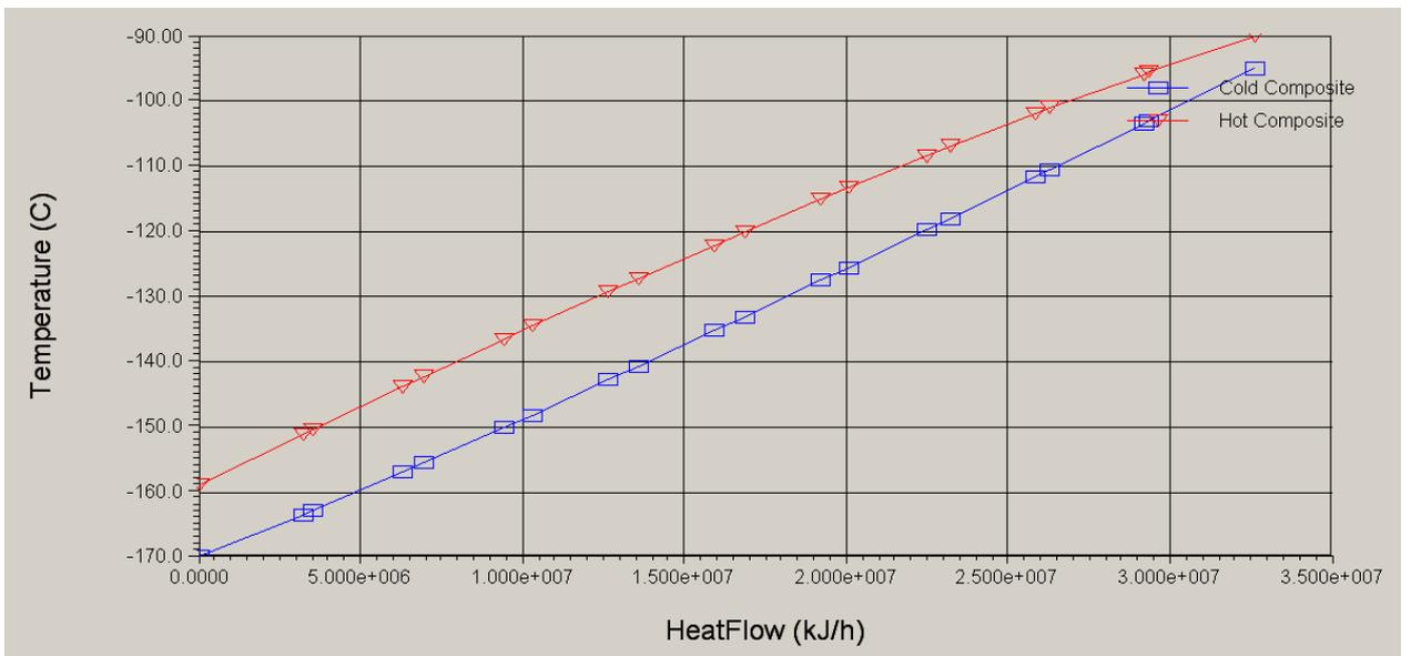
Composite curve for LNG heat exchanger LNG-2 (dual nitrogen expander process)
