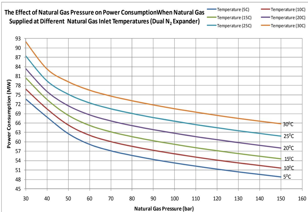
**Figure 67:** The effect of natural gas pressure on power consumption when natural gas supplied different temperatures (Dual nitrogen expander process).
