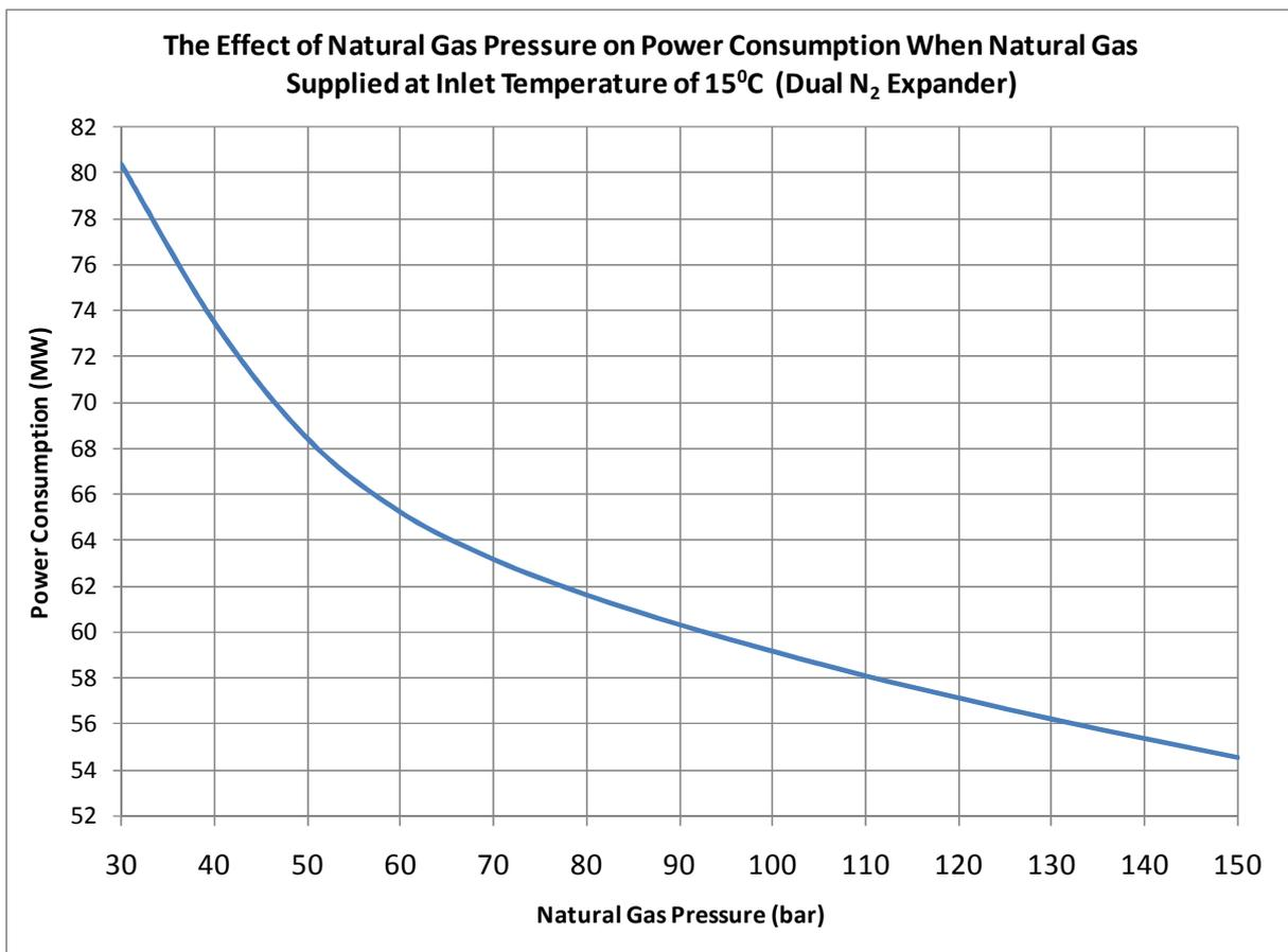
**Figure 66 :** The effect of natural gas pressure on power consumption when natural gas supplied at inlet temperature of 15°C (Dual Nitrogen Expander Process).
