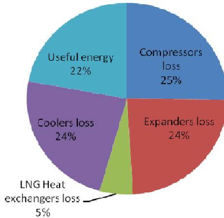
**Figure 71:** Exergy losses distribution at different component and useful effect (Dual N<sub>2</sub> expander process)
