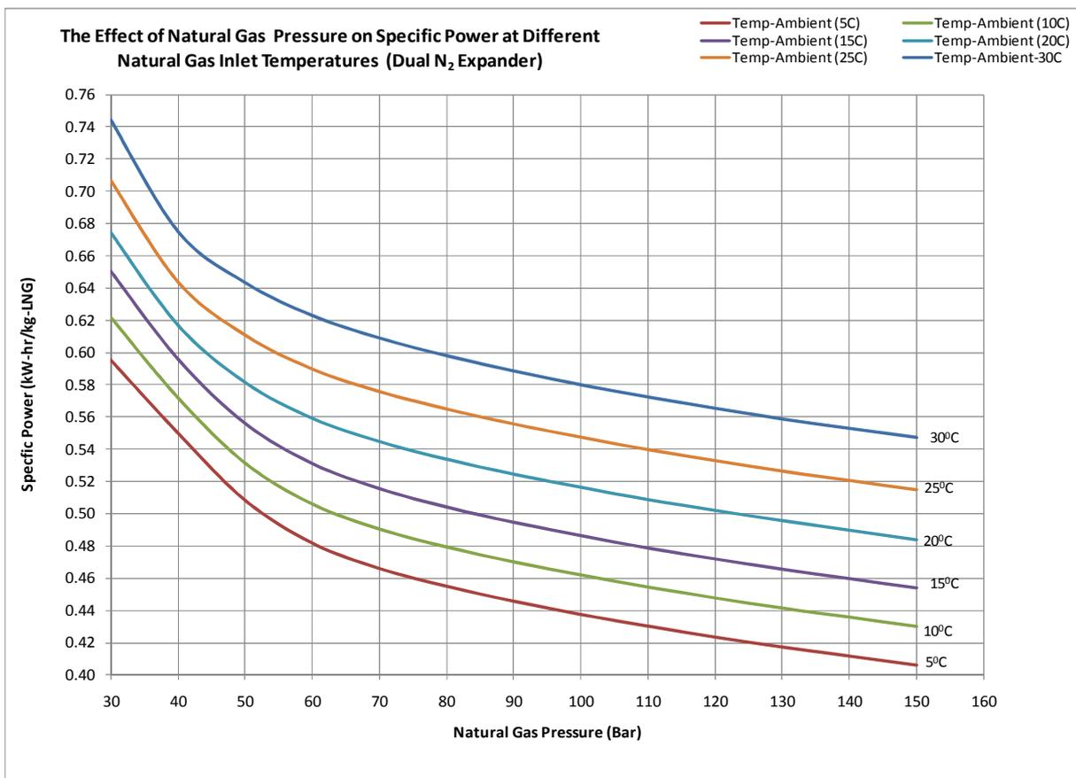
**Figure 65:** The effect of natural gas pressure on specific power when natural gas supplied at different inlet temperatures (Dual Nitrogen Expander Process).
