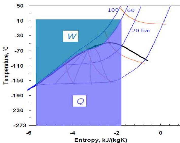
**Figure 4:**Temperature entropy diagram of natural gas with area showing heat removed (Q) and ideal work for reversible liquefaction process (W) (source [20])
