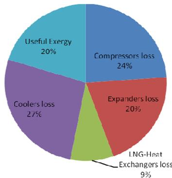
**Figure 57:** The distribution of exergy losses and useful effect in Niche LNG process
