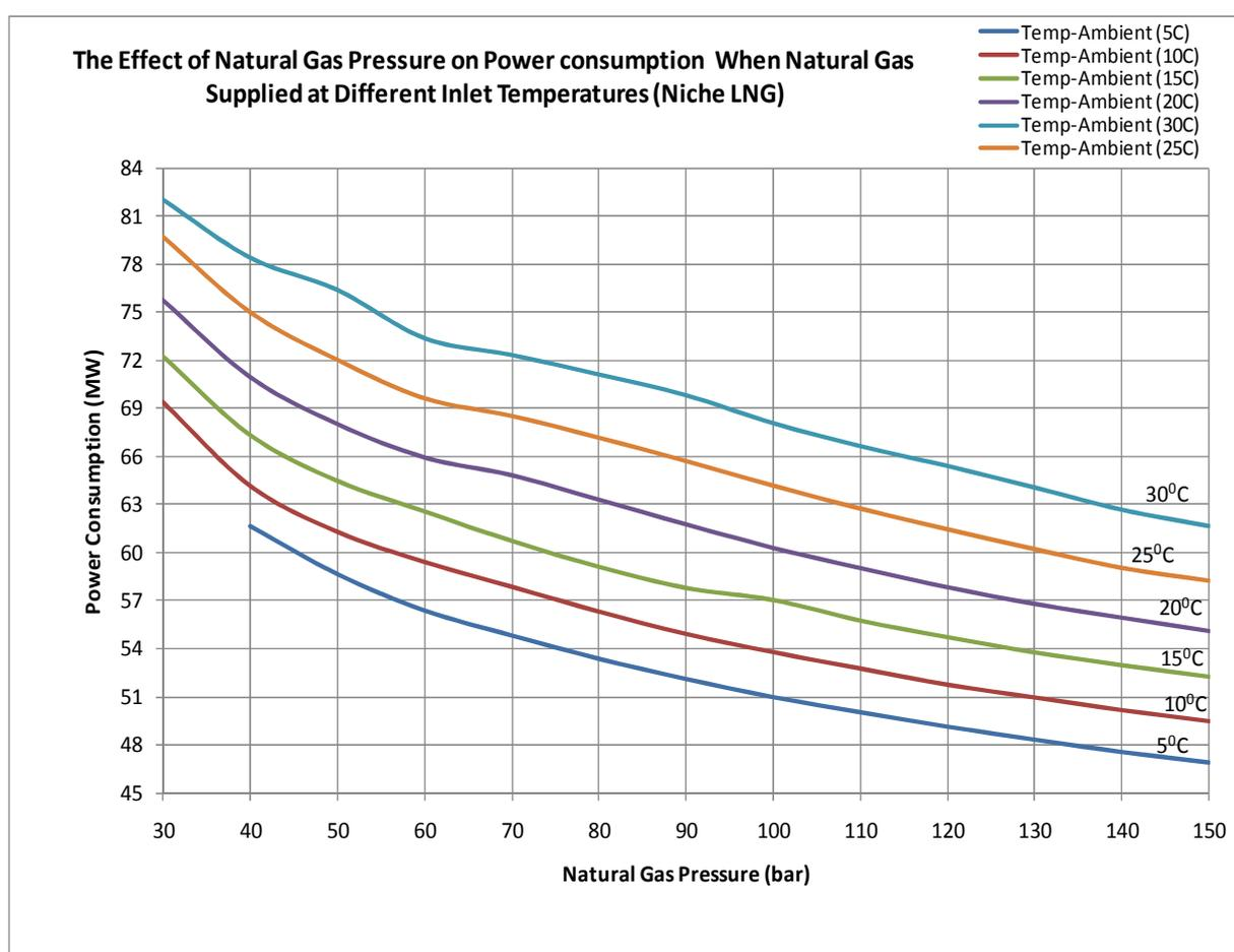
**Figure 53:** The effect of natural gas pressure on power consumption when natural gas supplied at different inlet temperatures (Niche LNG Process).
