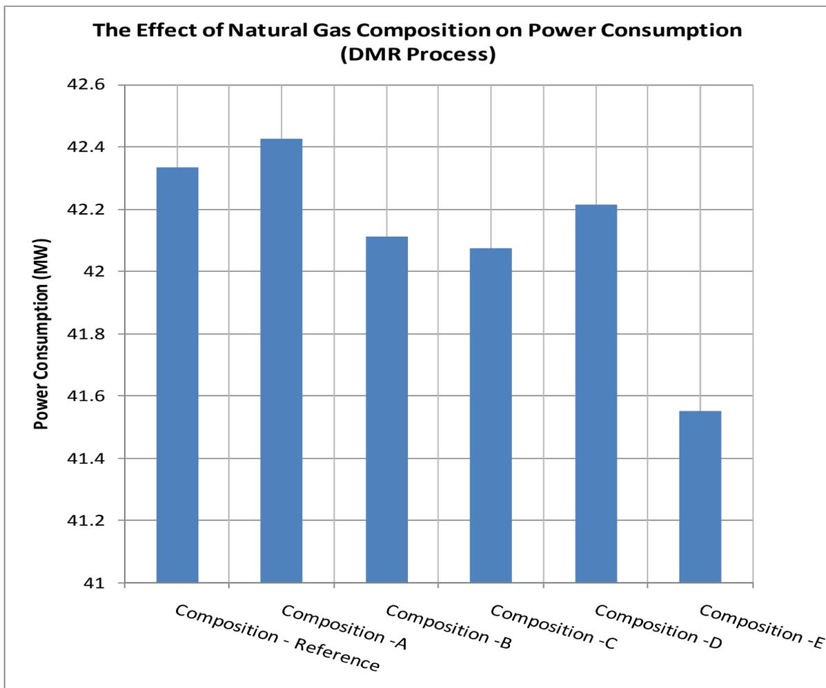
**Figure 41:** The effect of natural gas composition on power consumption (DMR Process)
