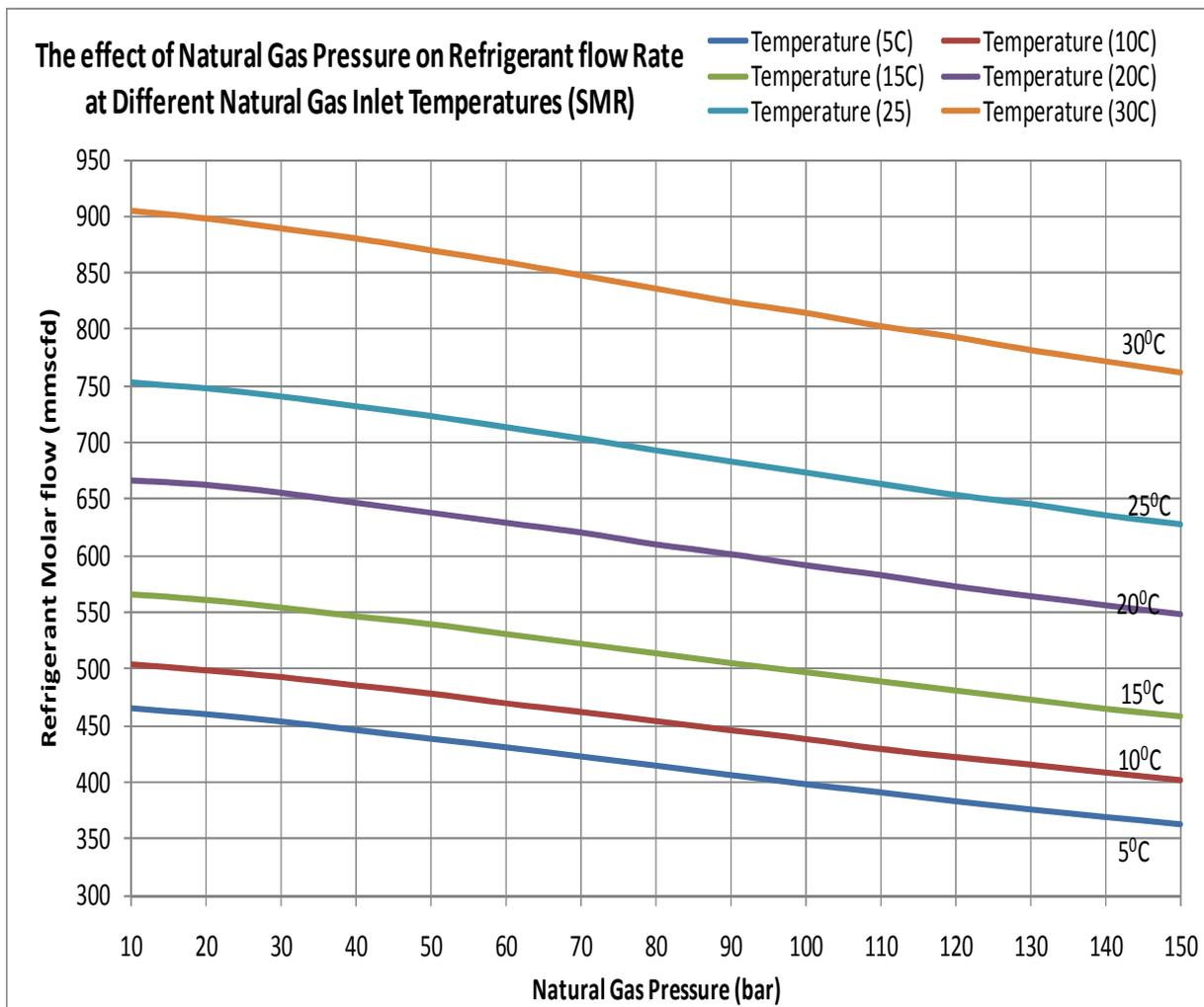
**Figure 21:** The effect of natural gas pressure on refrigerant flow when natural gas supplied at different temperatures (SMR-PRICO)
