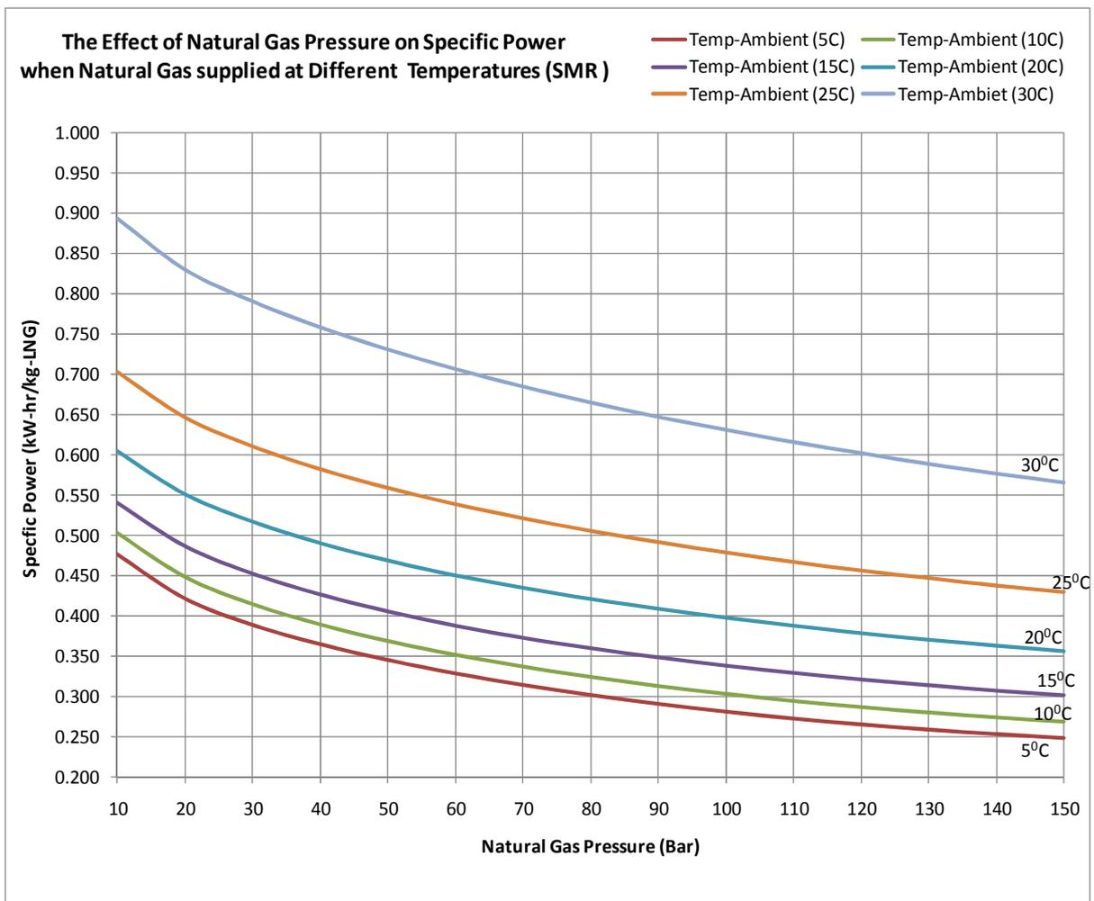
**Figure 17 :** The effect of natural gas pressure on specific power when natural gas supplied at different temperature (SMR-PRICO)
