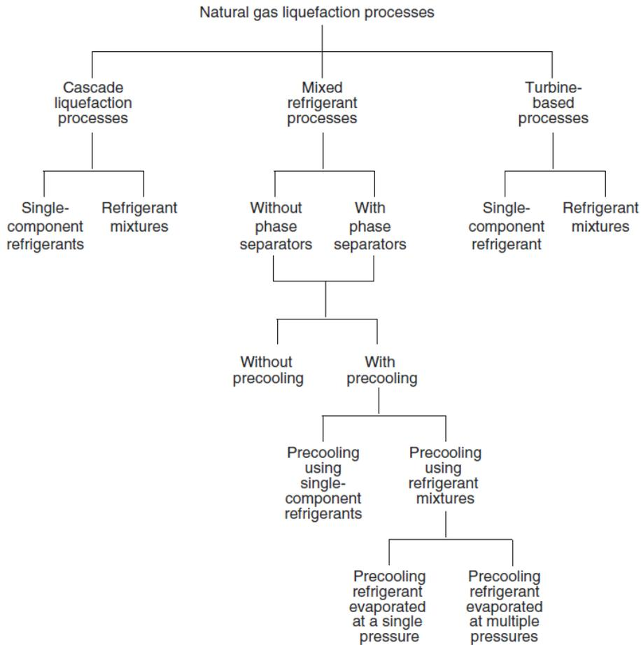
**Figure 2:** Classification of natural gas liquefaction processes (source [10])
