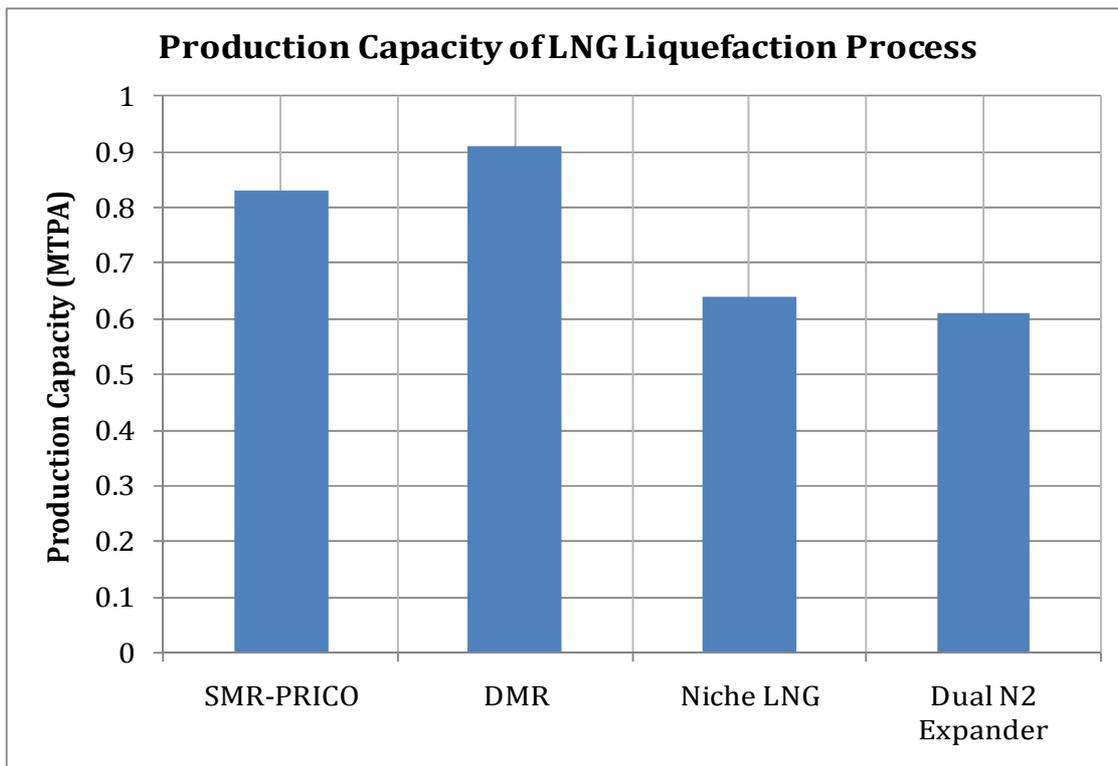
**Figure 76:** The comparison of production capacity of the proposed LNG processes for LNG FPSO
