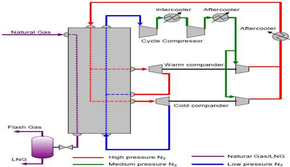
**Figure 8:** Diagram of dual nitrogen expander process (source [16])
