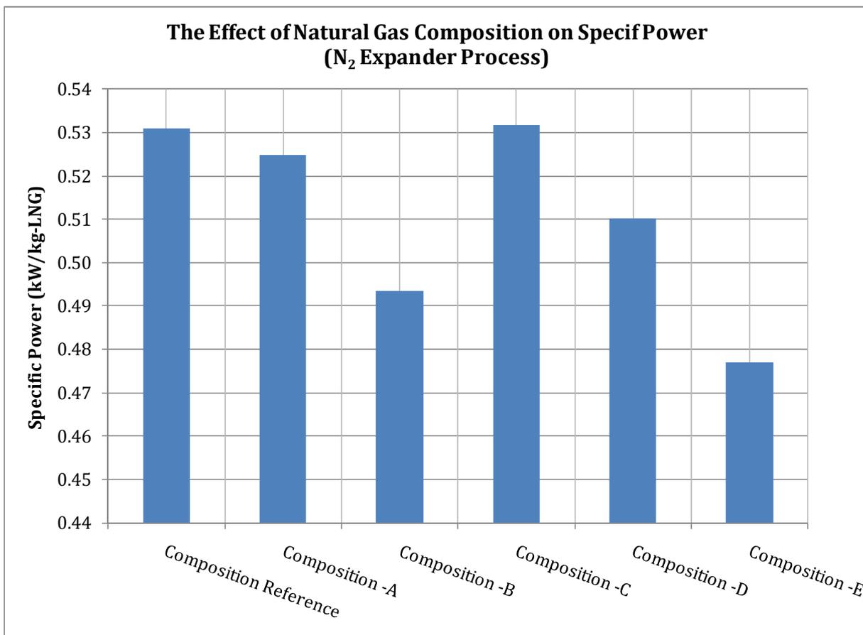
**Figure 68:** The effect of natural gas composition on specific power dual N<sub>2</sub> expander process
