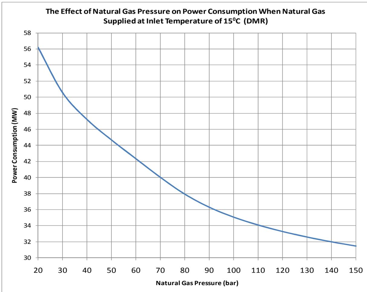
**Figure 36:** The effect of natural gas pressure on power consumption when natural gas supplied at 15°C (DMR Process)
