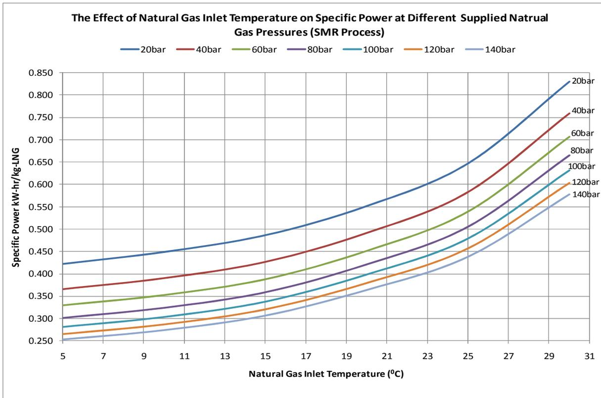
**Figure 11:** The effect of natural gas supply temperature on specific power when natural gas supplied at different pressures (SMR-PRICO)
