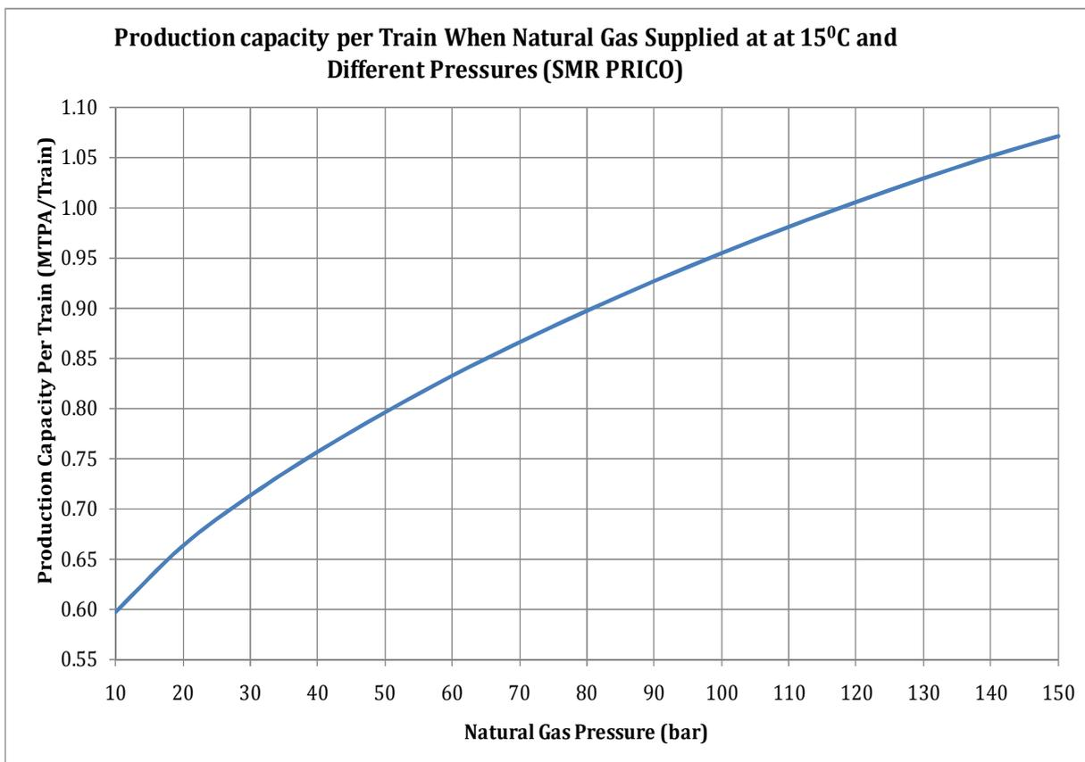
**Figure 26:** Production capacity of SMR process
