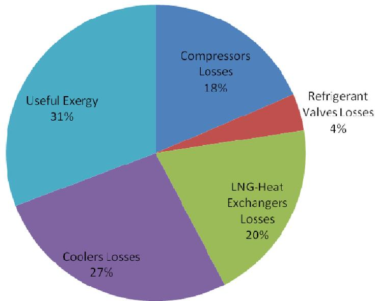
**Figure 43:** Distribution of exergy losses on different components and useful exergy (DMR)
