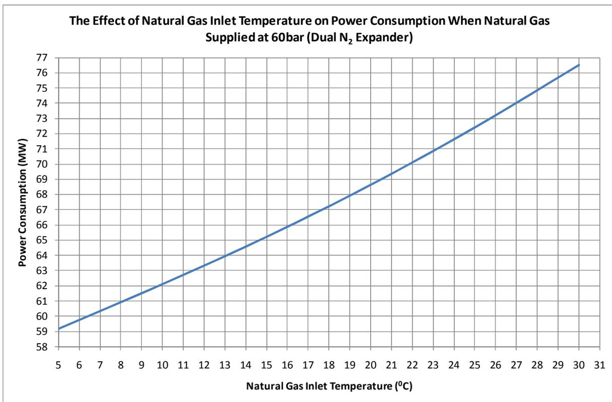
**Figure 62:** The effect of natural gas inlet temperature on power consumption when natural gas supplied 60bar (Dual Nitrogen Expander Process)
