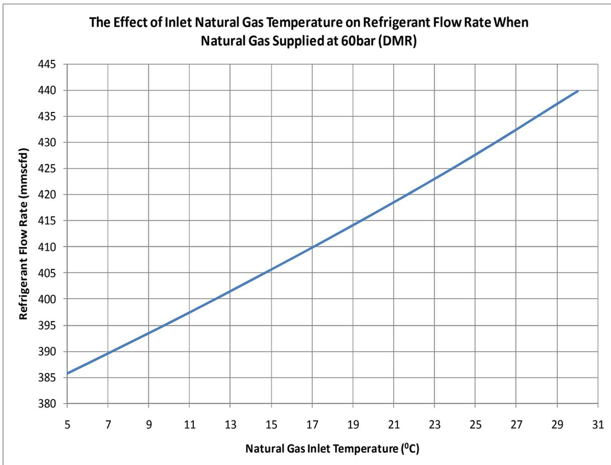
**Figure 32 :** The effect of natural gas inlet temperature on refrigerant flow rate when natural gas supplied at 60bar (DMR Process)
