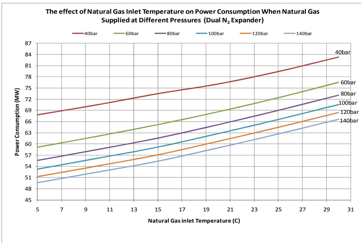
**Figure 63:** The effect of natural gas inlet temperature on power consumption when natural gas supplied at different pressures (Dual Nitrogen Expander Process).
