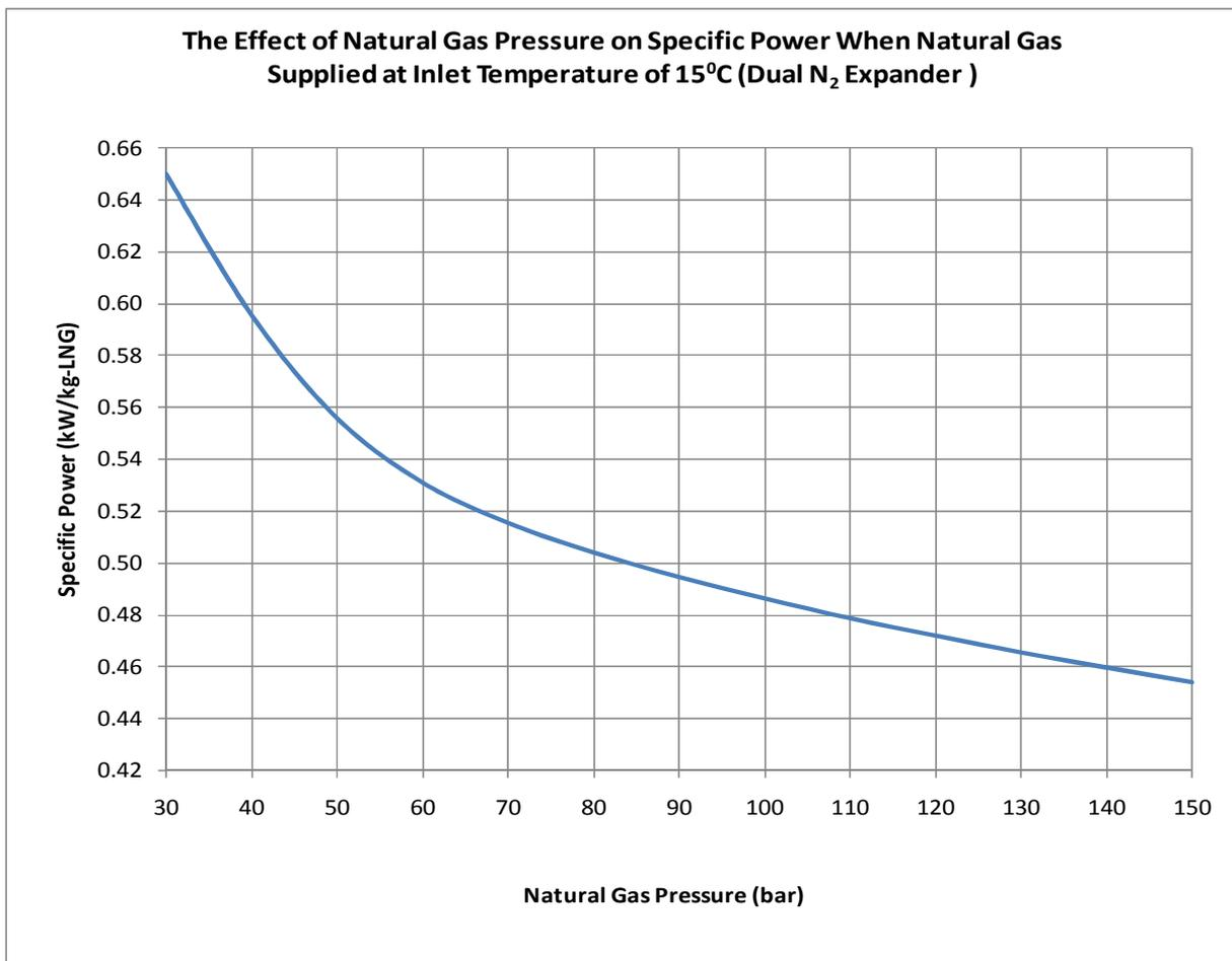
**Figure 64:** The effect of natural gas pressure on specific power when natural gas supplied at 15°C (Dual nitrogen expander process)
