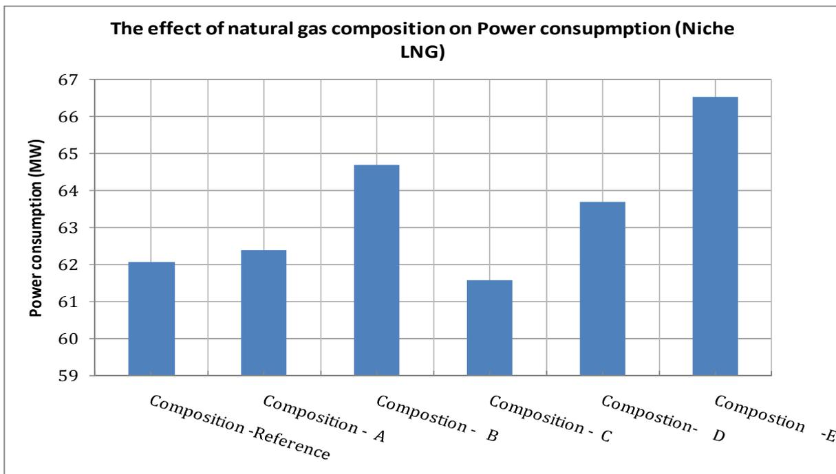
**Figure 55:** The effect of natural gas composition on power consumption (Niche LNG Process)
