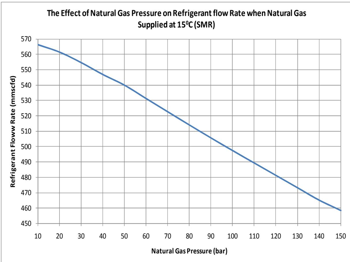
**Figure 20:** The effect of natural gas pressure on refrigerant flow rate when natural gas supplied at different temperatures (SMR-PRICO)
