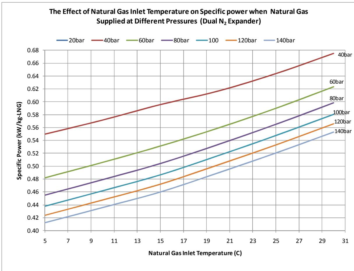
**Figure 61:** The effect of natural gas inlet temperature on specific power when natural gas supplied at different pressures (Dual Nitrogen Expander Process)
