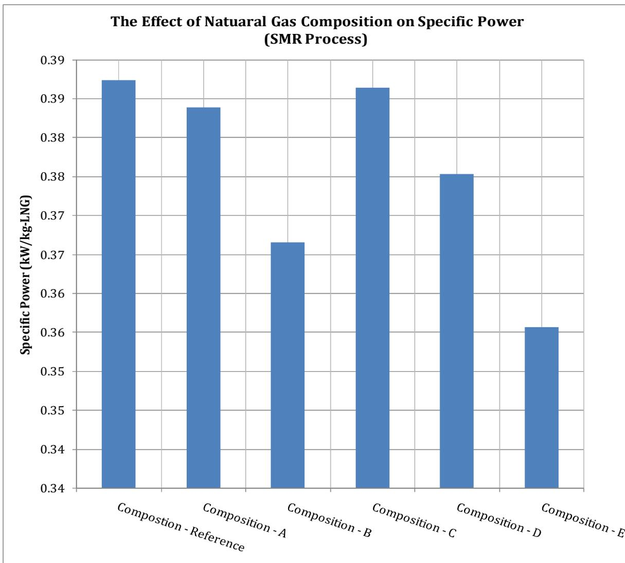
**Figure 22:** The effect of natural gas composition on specific power (SMR-PRICO)
