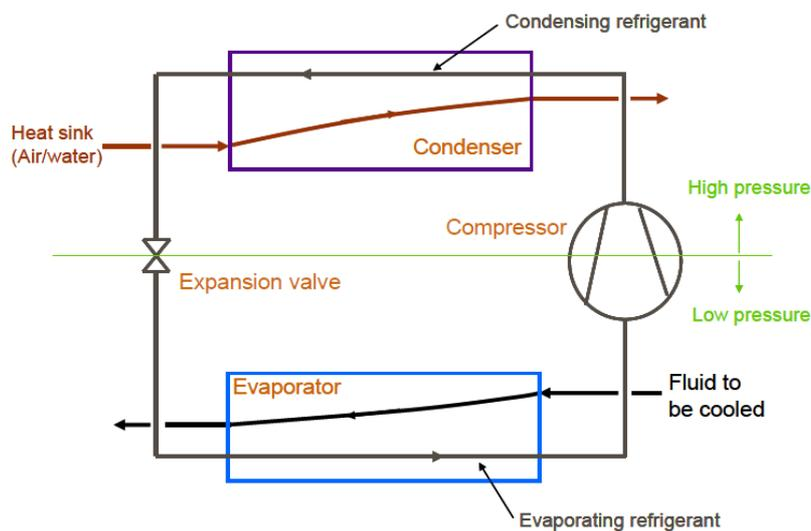
**Figure 3:** Flow diagram for single cycle refrigeration system (source [20])
