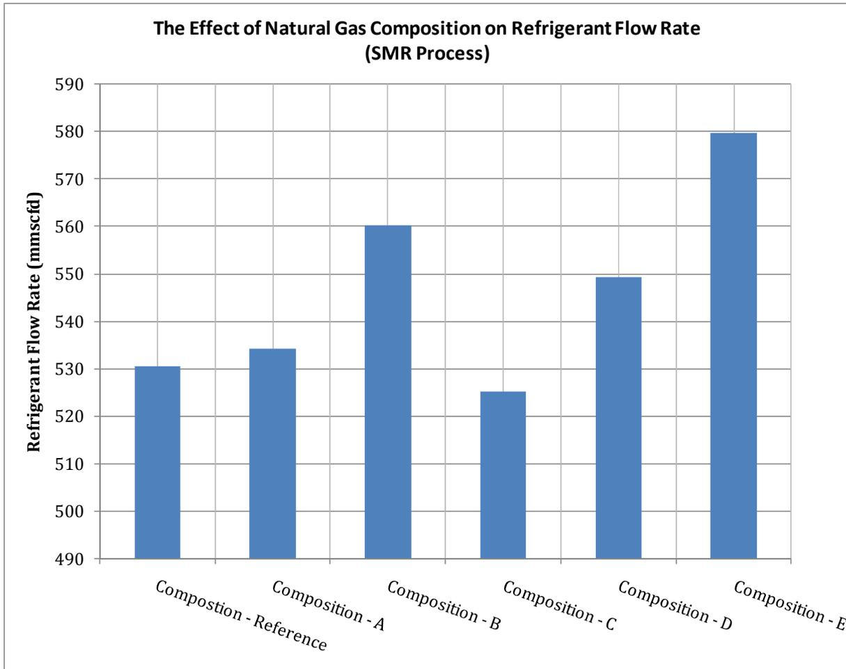
**Figure 24:** The effect of natural gas composition on refrigerant flow (SMR-PRICO)
