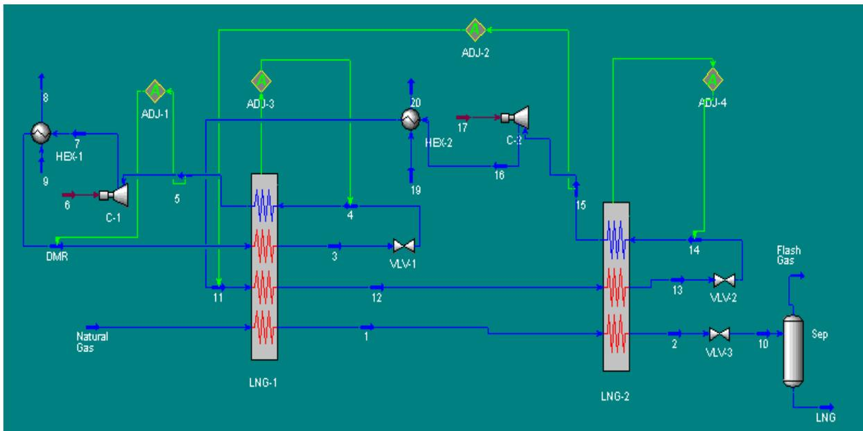
**Figure 27:** Process flow diagram for dual mixed refrigerant (DMR)
