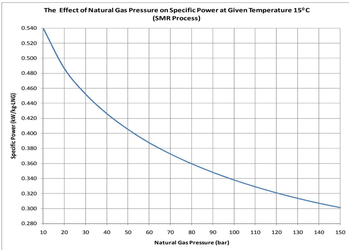
**Figure 16:** The effect of natural gas pressure on specific power when natural gas supplied at inlet temperature of 15°C (SMR-PRICO)
