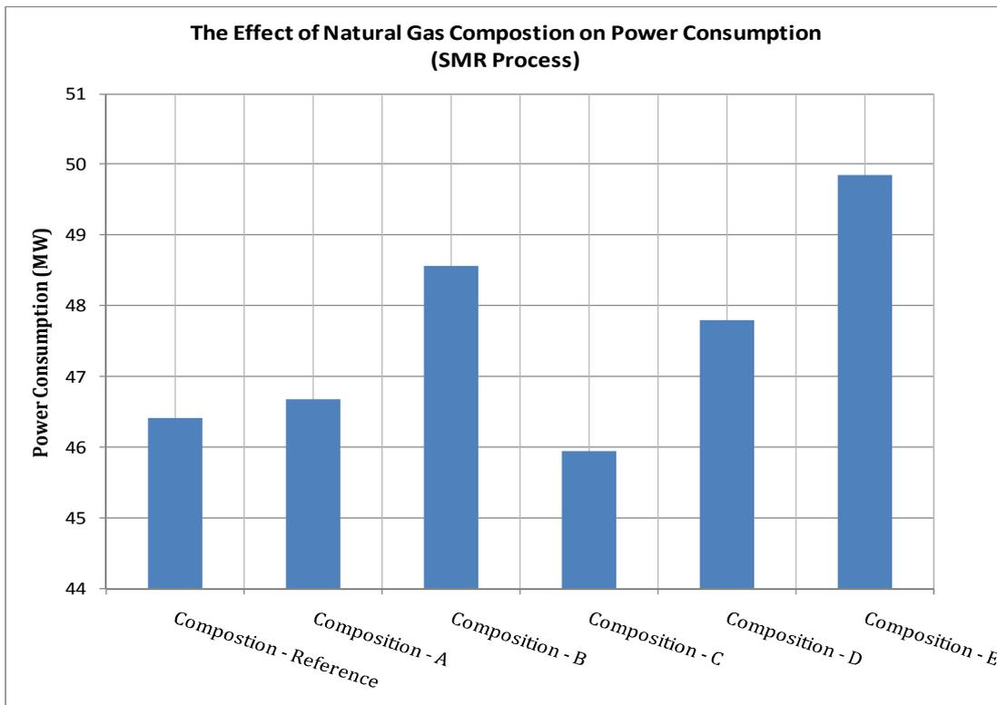
**Figure 23:** The Effect of natural gas composition on power consumption (SMR-PRICO)
