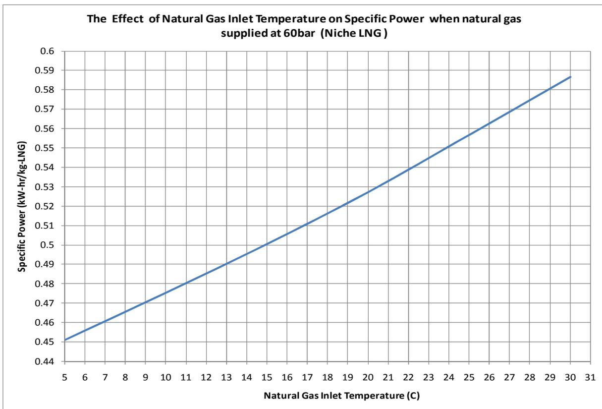
**Figure 46:** The effect of natural gas inlet temperature on specific power when natural gas supplied at 60bar (Niche LNG Process)
