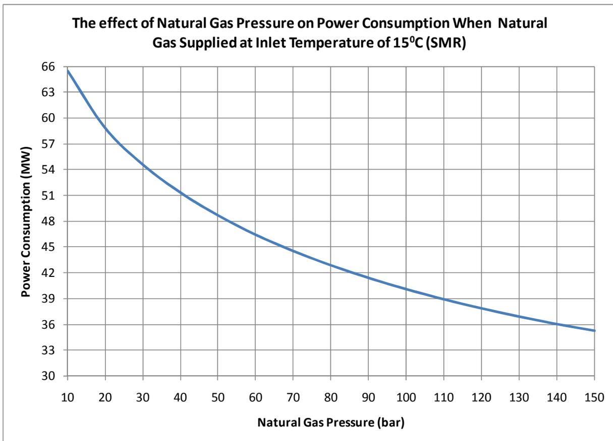
**Figure 18:** The effect of natural gas pressure on power consumption when natural gas supplied at inlet temperature of 15°C (SMR-PRICO)
