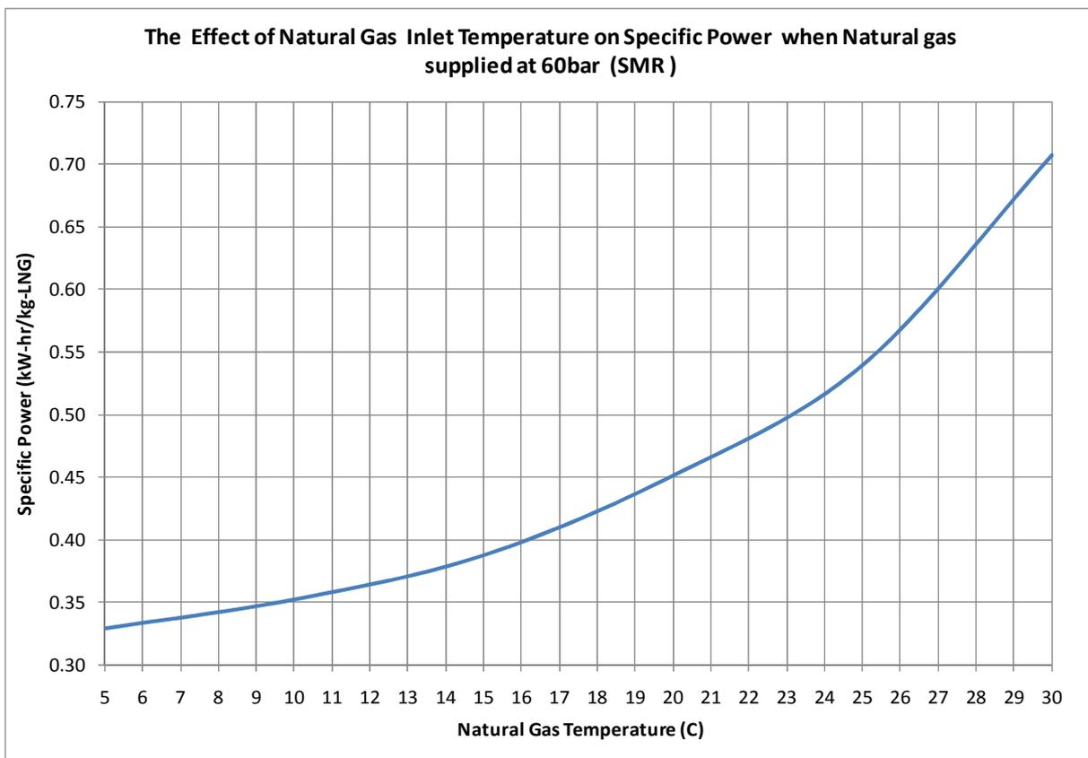
**Figure 10:** The effect of natural gas supply temperature on specific power when natural gas supplied at 60bar (SMR-PRICO)
