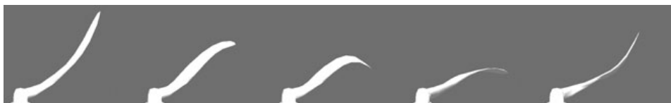
Figure 2.2: Example of a blade flutter mode over one period of oscillations on a wind turbine blade [2]
