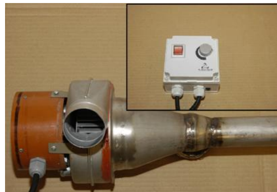
Figure 16 – 220 V radial air fan for sucking ambient air through the absorber. The appurtenant controllable motor inverter is shown in the inlay picture.
