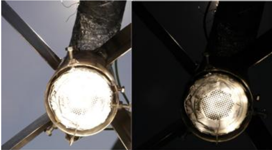
Figure 46 - Left: 40 mm SiC honeycomb absorber during testing. Right: Picture showing areas with highest flux.
