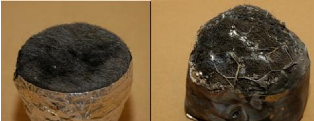
Figure 59 - Left: 70 mm flat absorber tested at TS2. Right: 80 mm 3D absorber tested at TS1.
