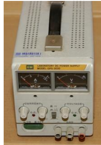
Figure 37 - DC power supply used for the tracking system and the air fan.
