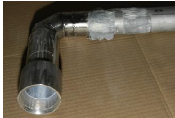
Figure 19 - Threaded welding socket at the receiver end of the 5 cm steel pipe for easy attachment and removal of different receivers.
