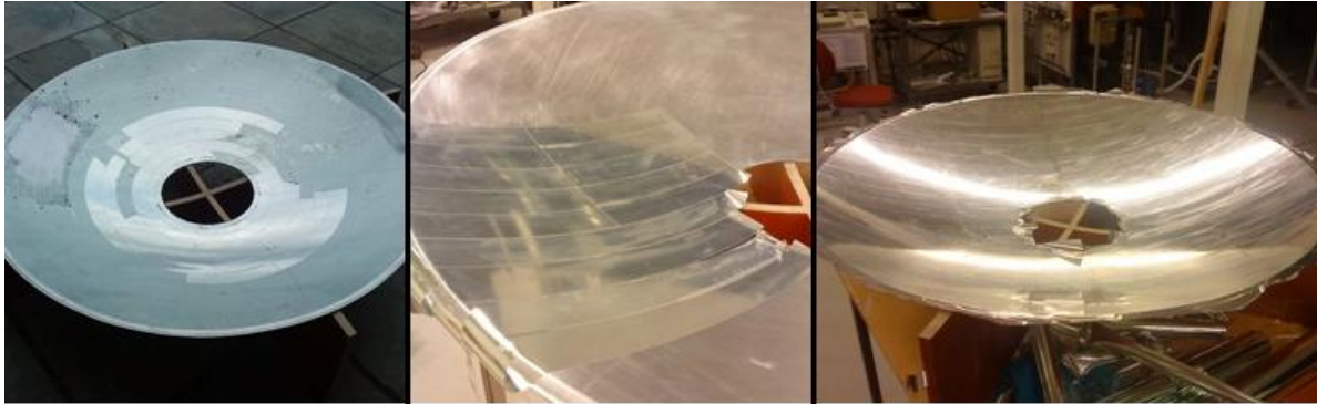
Figure 33- Replacement of reflective film to increase the dish's reflectance.
