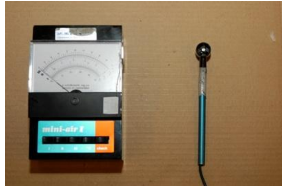
Figure 18 - Air velocity meter used at the fan outlet.
