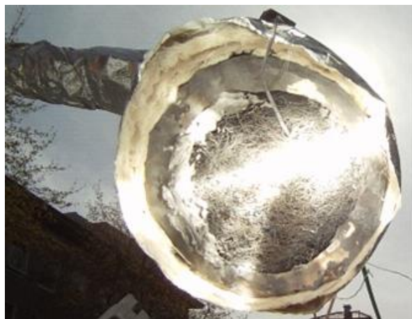
Figure 26 - Flat fiber absorber illuminated by reflected solar rays. More or less the same radiation profile at the absorber was observed when tested indoors.
