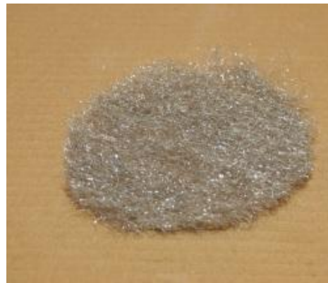
Figure 20 – Sample of stainless steel fiber mesh used to form the fiber mesh absorber.
