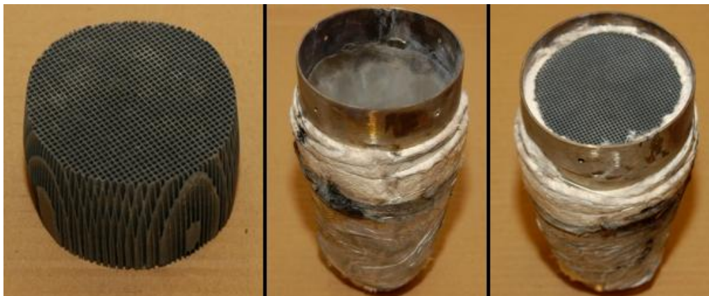
Figure 30 - Assembly of honeycomb receiver
