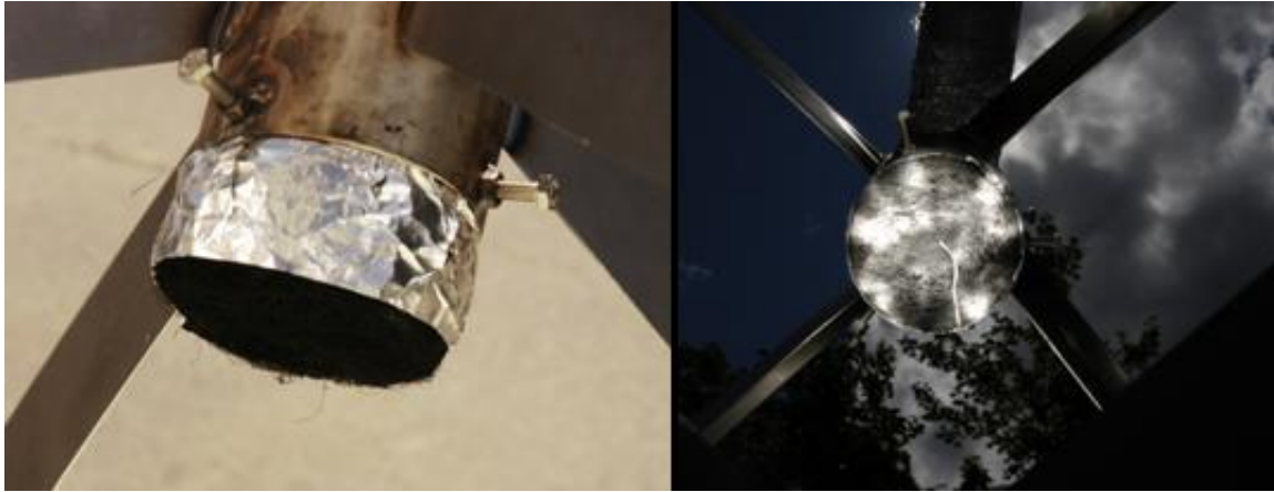
Figure 44 – Left: 70 mm fiber absorber positioned and ready for testing. Right: Underexposed picture of the absorber while illuminated.
