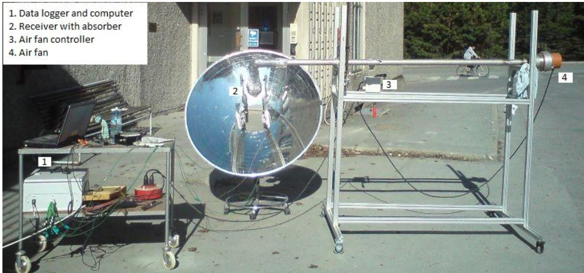
Figure 12 - Picture of Test Setup 1 during operation.
