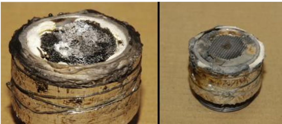
Figure 60 - Left: 40 mm foam absorber after testing. Right: 40 mm honeycomb after testing.
