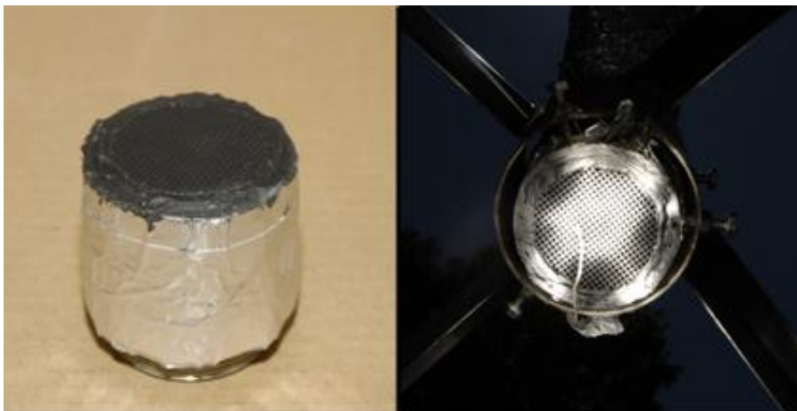
Figure 45 - Left: 50 mm SiC honeycomb absorber before testing. Right: Underexposed picture of absorber during testing.
