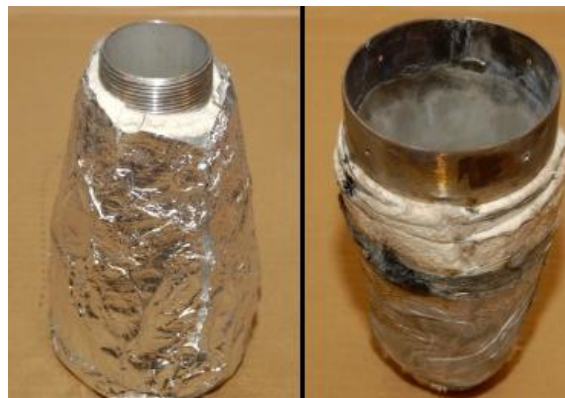
Figure 22 – Receiver used to house and support the absorber during testing in Test Setup 1.
