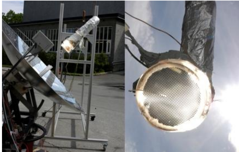
Figure 31 - Left: Parabolic dish on a solar tracking system. Right: Large un-illuminated areas on absorber.
