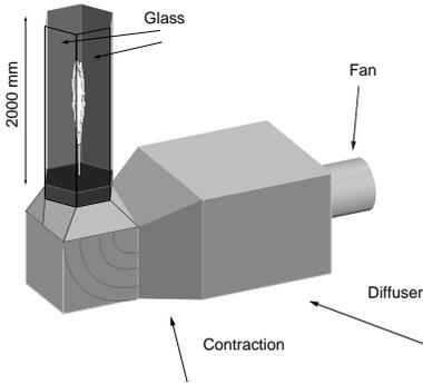
Figure 1: Sketch of the test facility
