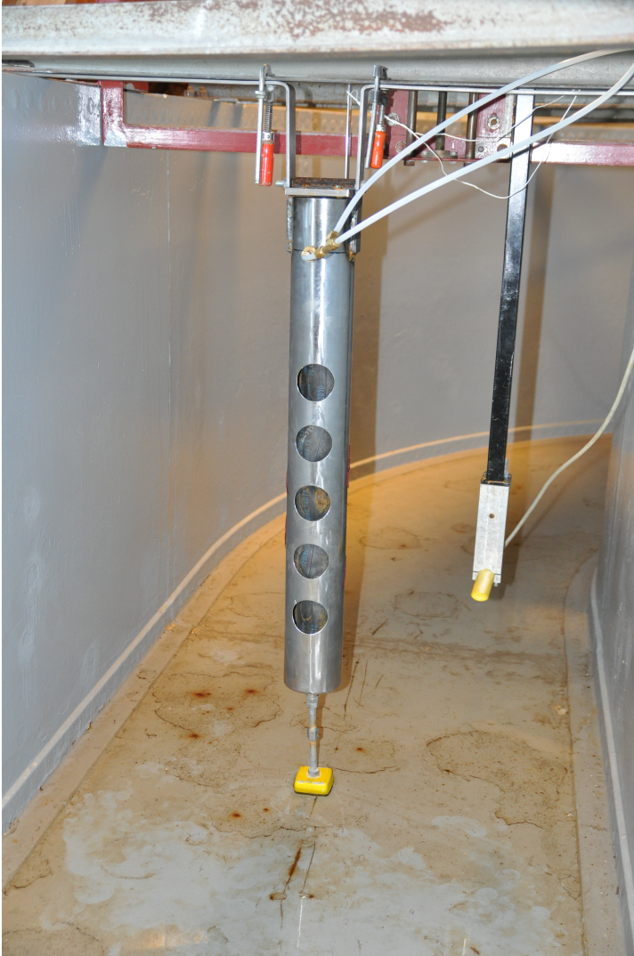
Figure 4.1: An upstream view of the rig, with the velocity sensor on flow right.
