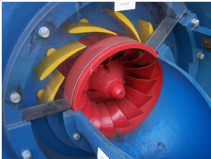
Figure 2.1: Francis turbine cut-away. Guide vanes (yellow) are at full opening. The inlet of the draft tube can be seen in the lower right corner. Spiral casing and stay vanes upstream of guide vanes (not clearly visible). Source: Wikimedia Commons[1]
