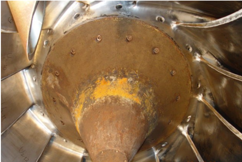
Figure 4.4: Cavitation on the hub
