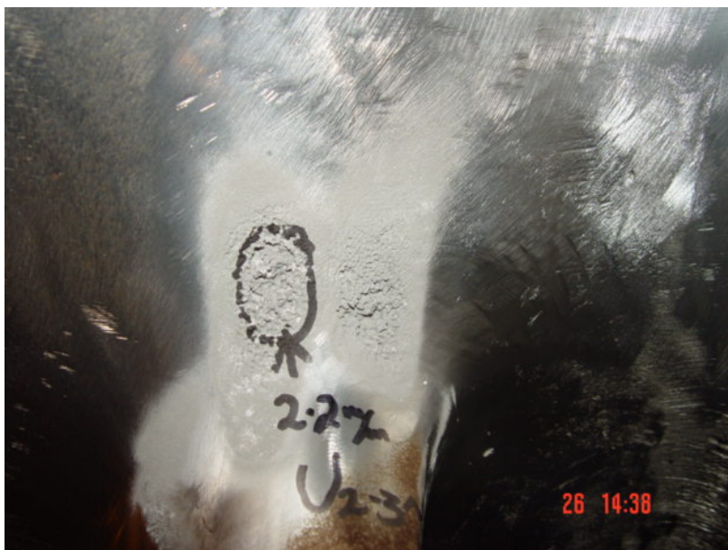
Figure 4.5: Cavitation on the trailing edge and the outer ring
