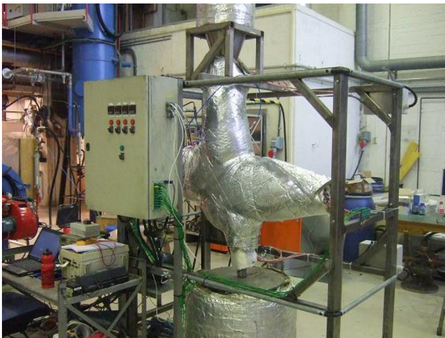
Figure 3.19: Second layer of insulation at test #2, L10-56 test rig.
