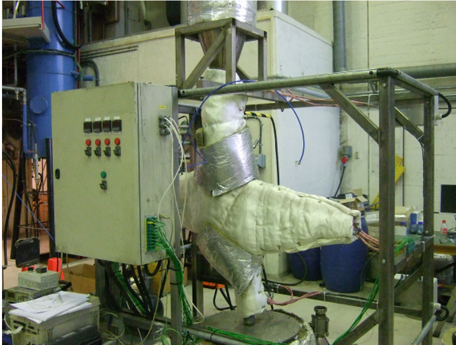
Figure 3.18: Filter during heating test #1, L10-56 test rig.
