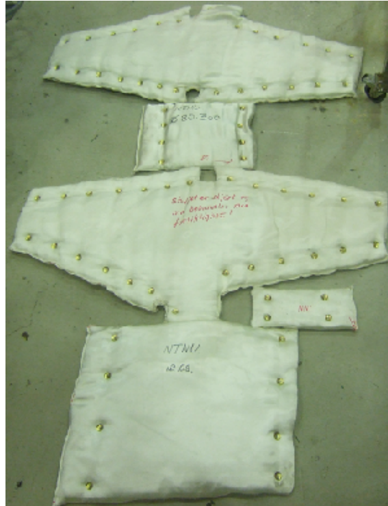
Figure 3.15: Specially fitted insulation.
