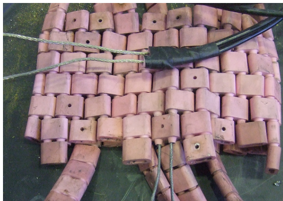
Figure 3.14: L10-56 heating cables.
