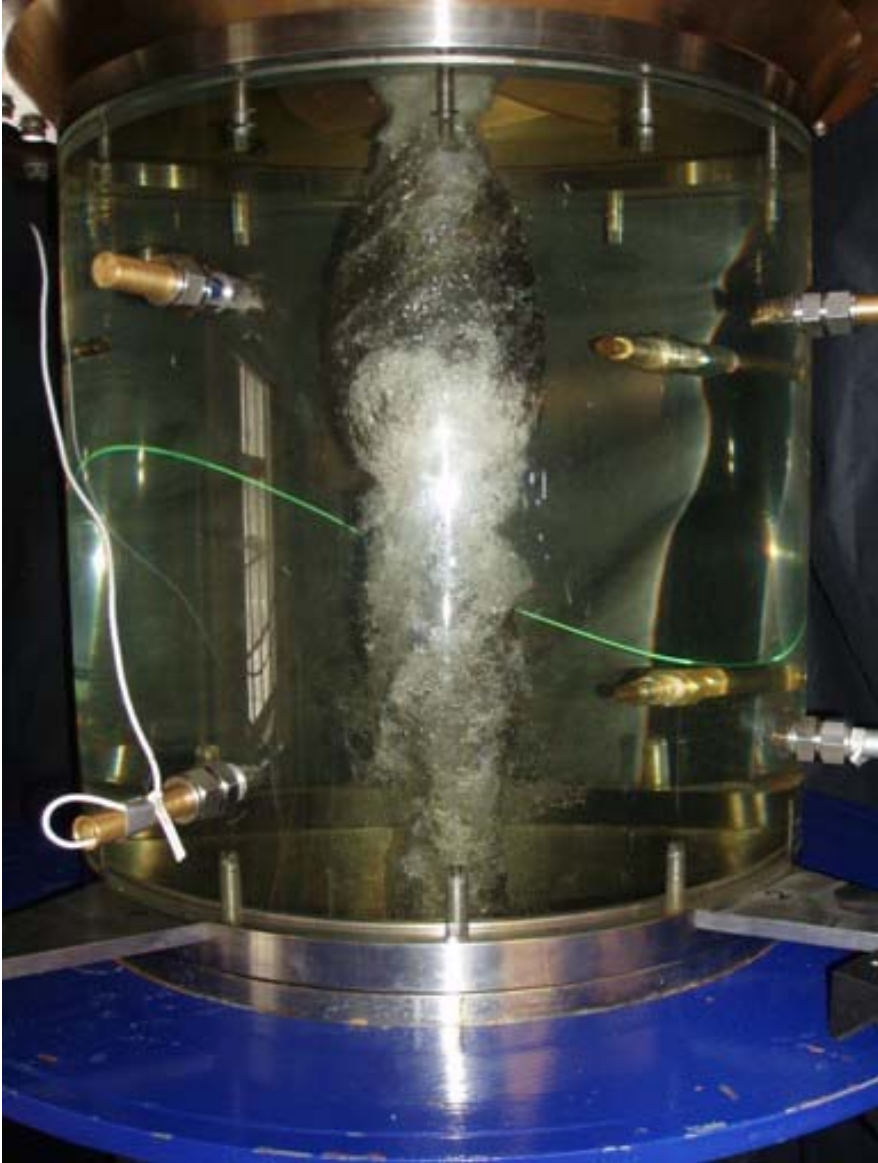
Figure 9-8. n_{ED}=0.165 q_{ED}=0.175 , \alpha=11^\circ . Overload
