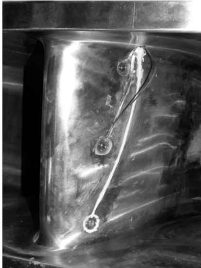
Figure 4 - Inlet pressure sensors during installation
