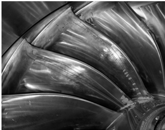
Figure 2 - Strain gauges and pressure covering cables transducers with cables fixed, before covering
