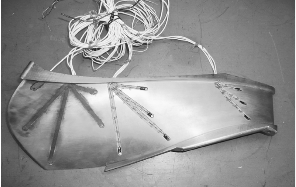
Figure 2 – Pressure transducers in the NTNU runner, during installation.
