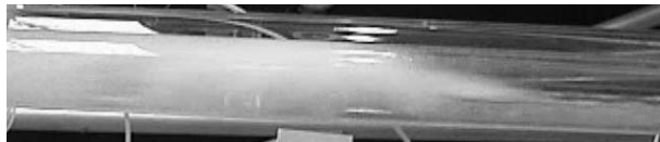
Figure 5: An individual slug: peaks from the 3 rd holdup time trace H3, the 4 th holdup time trace H4, and the pressure time trace P overlapped (top plot) and corresponding video snapshot (bottom). U_{sl} = 0.52 m/s, U_{sg} = 3.63 m/s, and inclination of -1 degrees.
