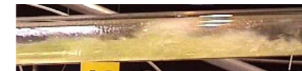
Figure 6: Overlapped signals for liquid fraction time trace 3 and 4 and the pressure time trace and the matching video snapshot for the 0 degrees, U_{sg} = 5.89 m/s and U_{sl} = 0.17 m/s. The pressure signal is multiplied by a factor of 10 so that it can be seen on the same plot as the liquid fraction.
