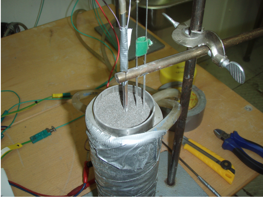
Figure 9.2.: Test Rig - New Cylinder Filled with Sand
