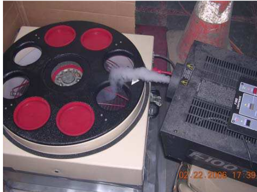
Figure 5.4: “Theatrical” smoke induction into fan inlet [Gupta & Woods 2007].
