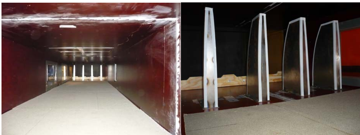
Figure 13: Barrier, spires and roughness fetch installed in the wind tunnel.
